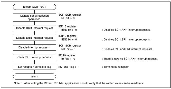
Figure 5.11 SCI1 Receive Data Full Interrupt Handler
