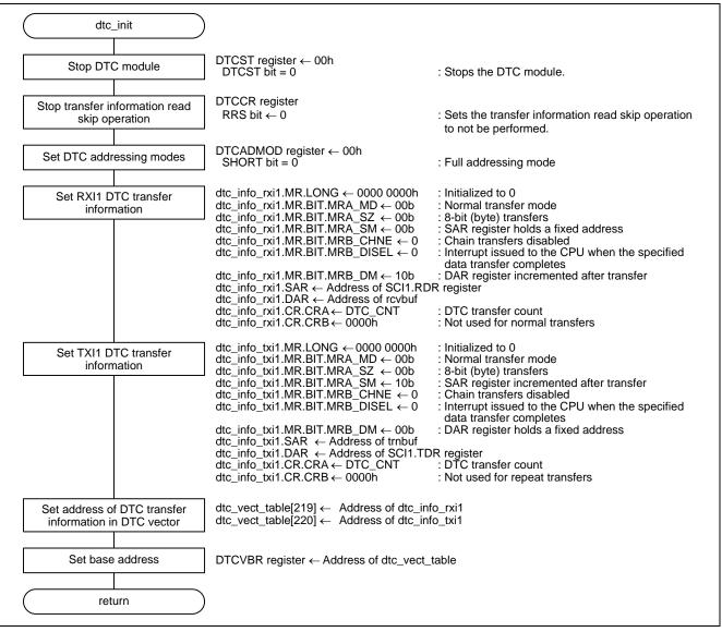
Figure 5.8 DTC Initialization
