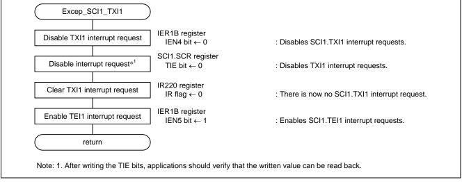
Figure 5.12 SCI1 Transmit Data Empty Interrupt Handler
