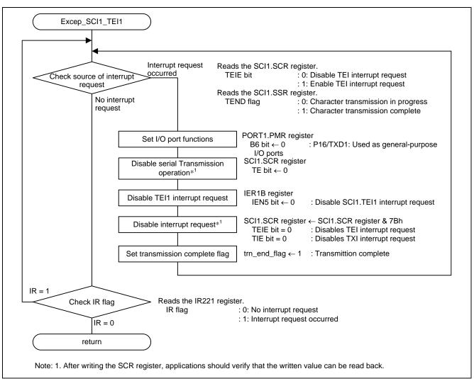
Figure 5.13 SCI1 Transmission Complete Interrupt Handler
