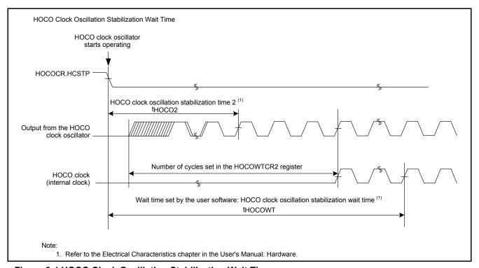
Figure 3.4 HOCO Clock Oscillation Stabilization Wait Time
