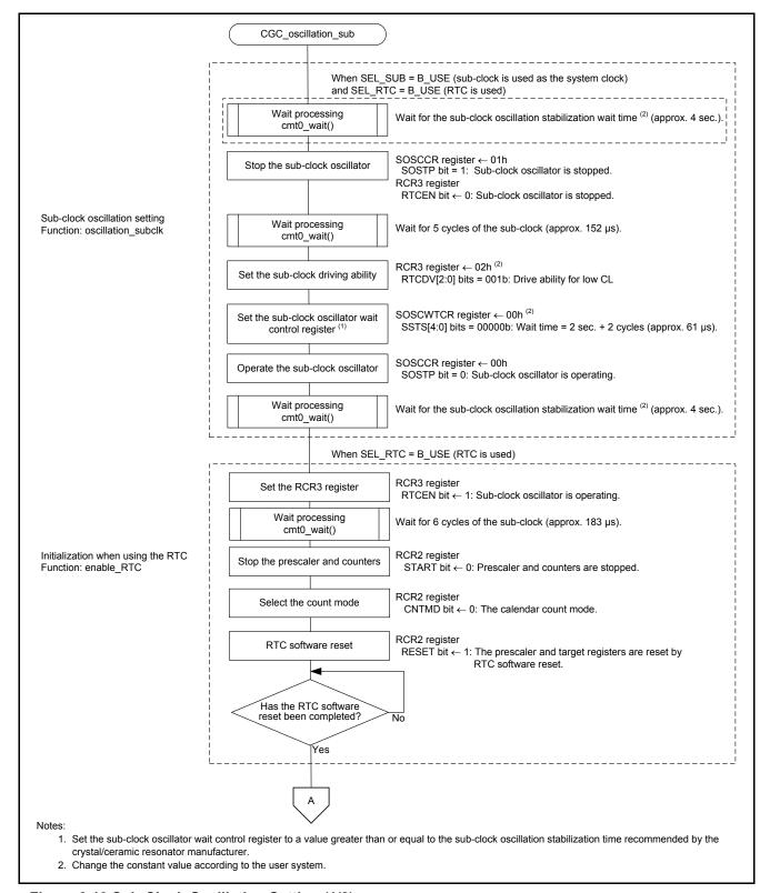
Figure 3.13 Sub-Clock Oscillation Setting (1/2)
