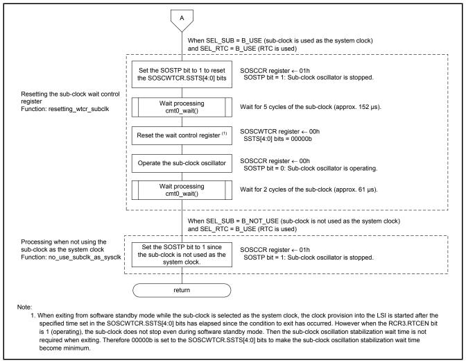
Figure 3.14 Sub-Clock Oscillation Setting (2/2)
