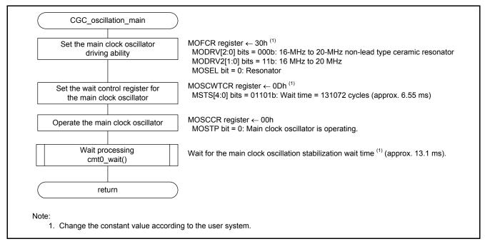
Figure 3.10 Main Clock Oscillation Setting
