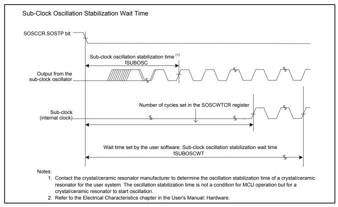
Figure 3.3 Sub-Clock Oscillation Stabilization Wait Time
