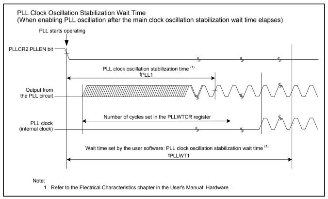
Figure 3.2 PLL Clock Oscillation Stabilization Wait Time
