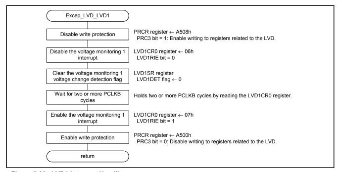
Figure 5.20 LVD1 Interrupt Handling
