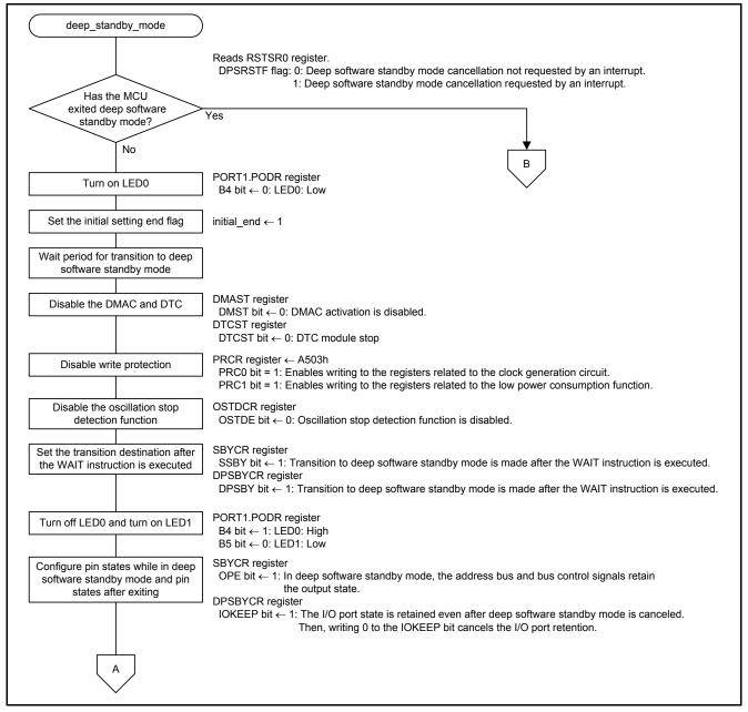
Figure 5.12 Transition to Deep Software Standby Mode (1/3)
