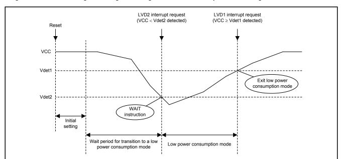
Figure 5.6 shows the Timing of Entering and Exiting a Low Power Consumption Mode Using the LVD.
