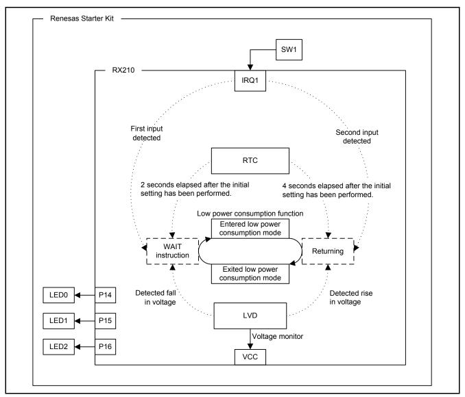
Figure 1.1 Block Diagram
