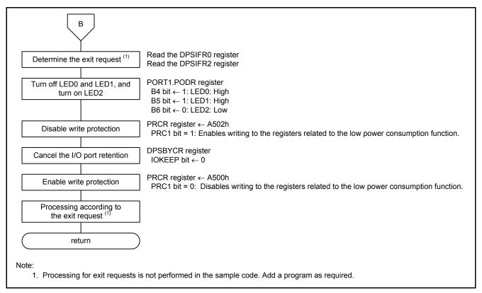
Figure 5.14 Transition to Deep Software Standby Mode (3/3)
