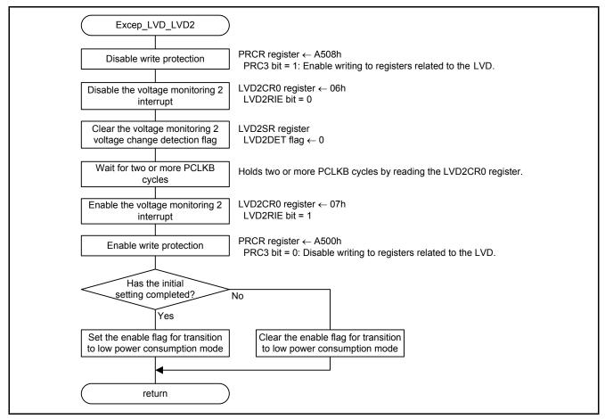
Figure 5.21 LVD2 Interrupt Handling
