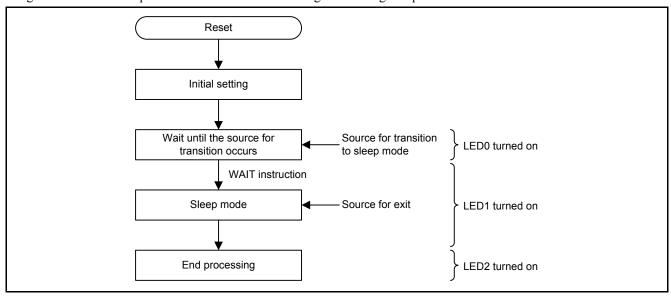
Figure 5.1 Operation Overview when Entering and Exiting Sleep Mode
