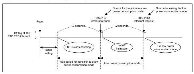
Figure 5.5 Timing of Entering and Exiting a Low Power Consumption Mode Using the RTC
