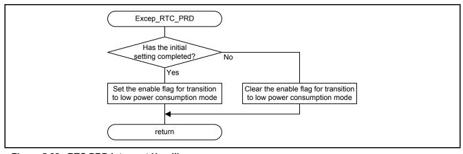
Figure 5.22 RTC.PRD Interrupt Handling
