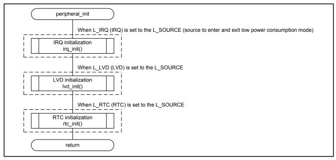
Figure 5.9 Peripheral Function Initialization
