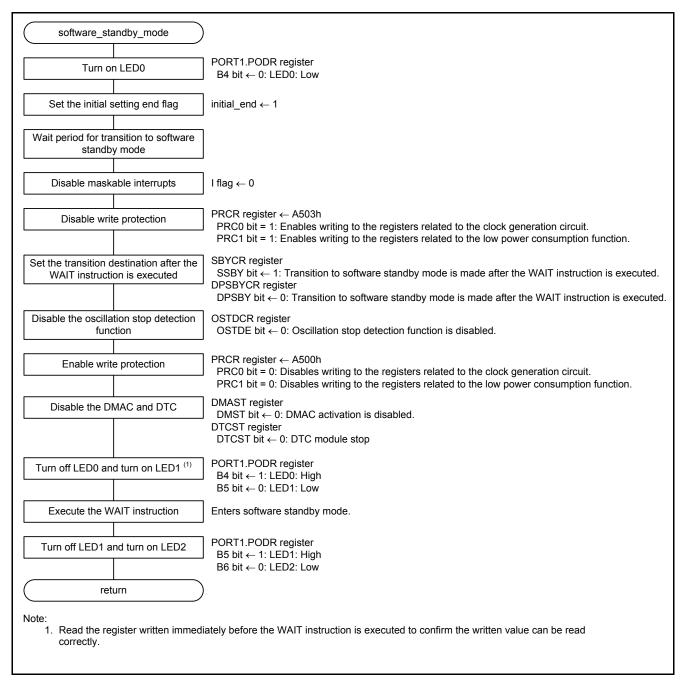
Figure 5.11 Transition to Software Standby Mode
