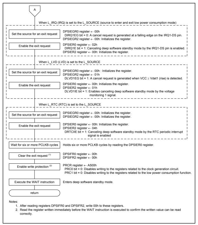
Figure 5.13 Transition to Deep Software Standby Mode (2/3)
