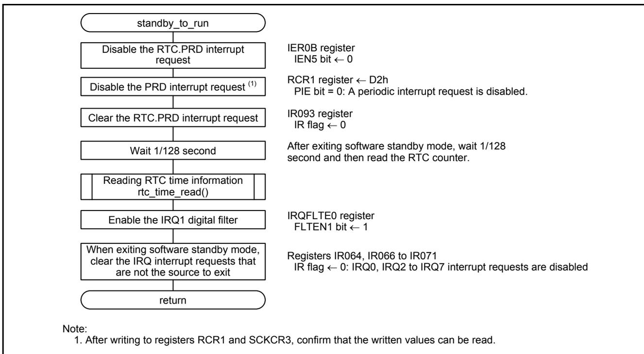
**Figure 5.12 Exiting Software Standby Mode**
