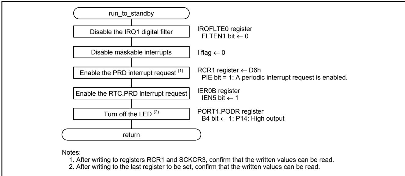
**Figure 5.11 Preparation to Enter Software Standby Mode**
