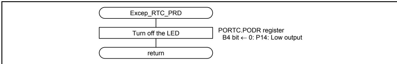
**Figure 5.13 PRD Interrupt Handling**
