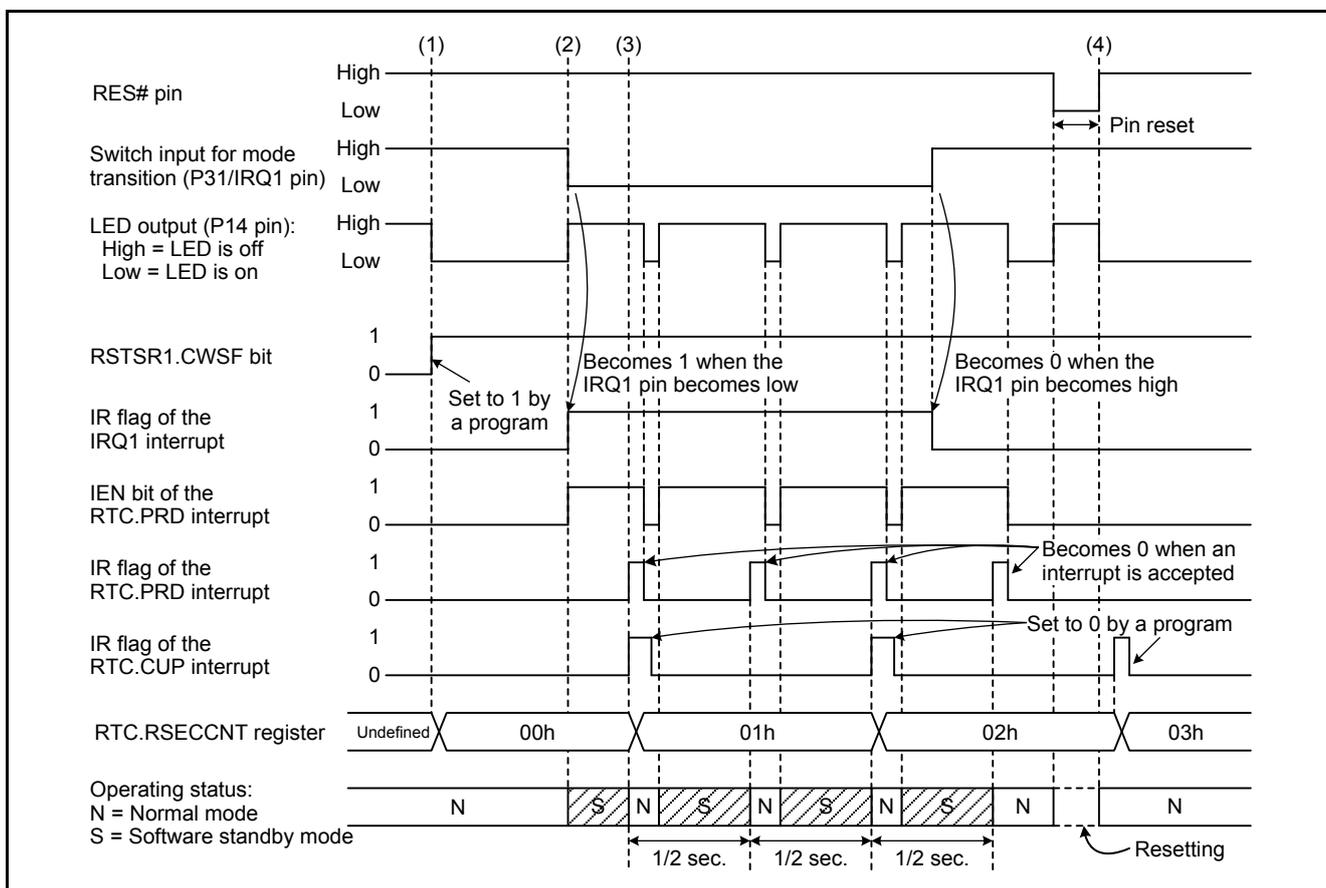
**Figure 5.1 Timing Diagram**
