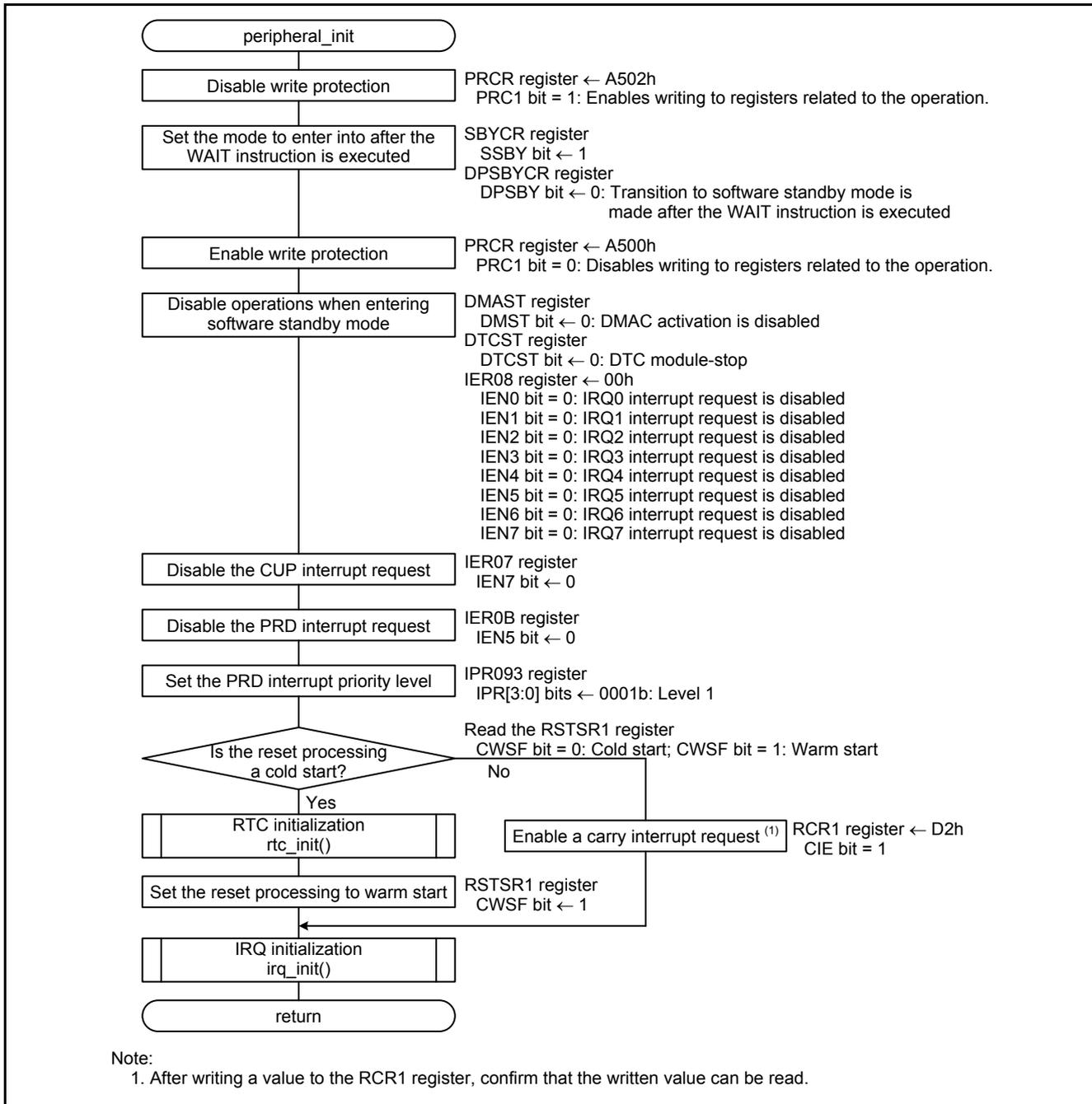
**Figure 5.7 Peripheral Function Initialization**
