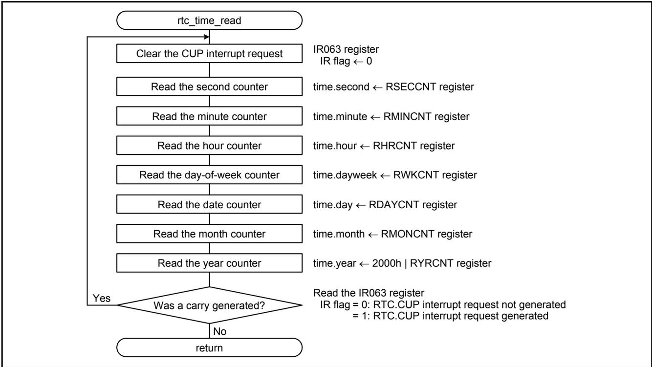
**Figure 5.10 Reading RTC Time Information**
