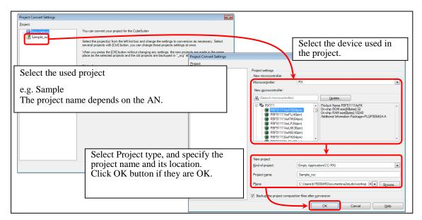
Figure 10-1 Using the e<sup>2</sup> studio project with CS+
