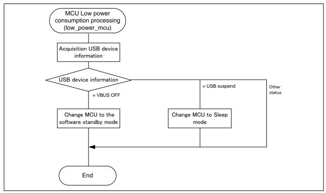
Figure 7-3 Flowchart of MCU Low Power Consumption Processing
