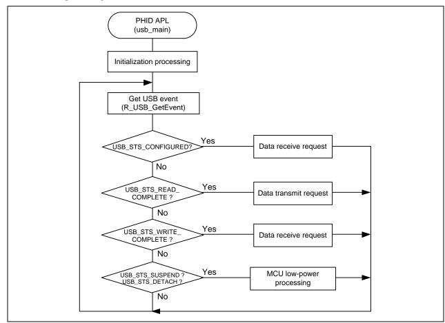
Figure 7-2 Main Loop Processing (Echo mode)
