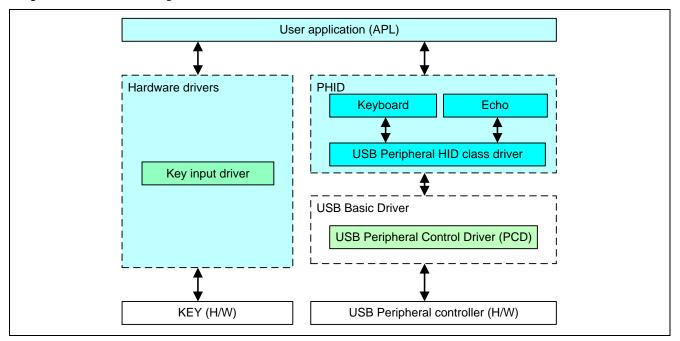
Figure 2-1 Source Code Block Diagram
