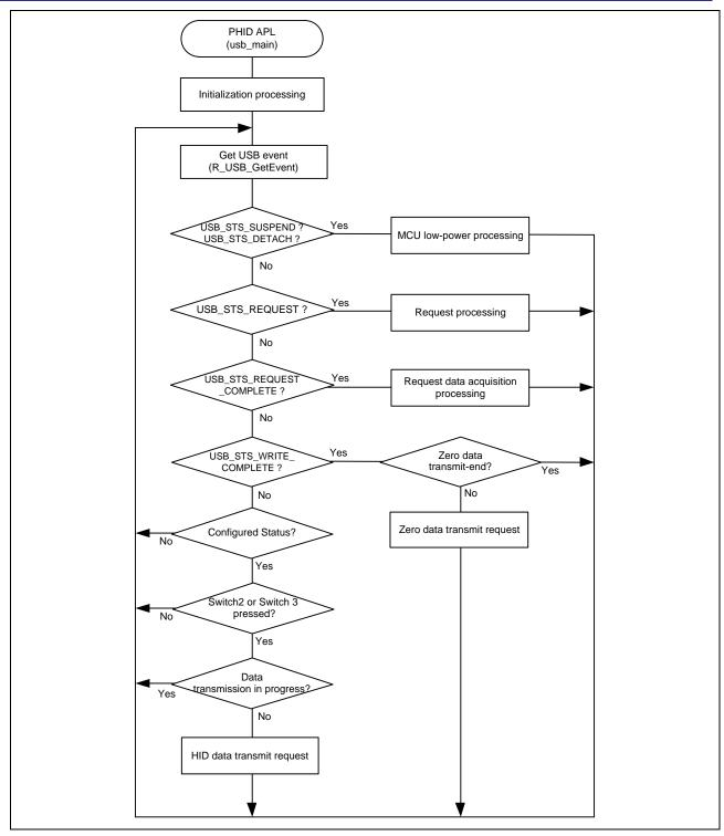
Figure 7-1 Main Loop Processing (Keyboard mode)
