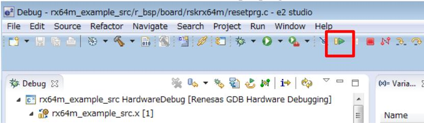
6) As stopping at the first line of main(), click Resume icon again. The sample program execution is restarted. Sampling rate conversion operation is started and PCM data after conversion is stored in PCM read buffer.
