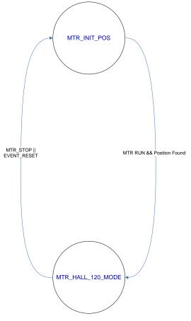
Figure 4: Motor State Diagram, HALL
