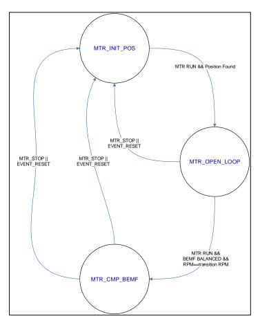
Figure 3: Motor State Diagram, Sensorless
