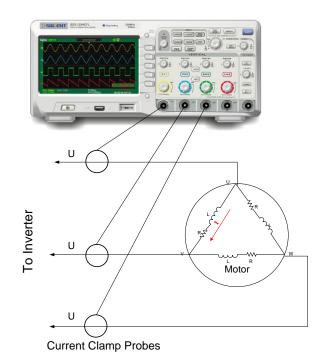
Figure 6: Motor current monitoring set-up
