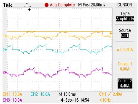
Figure 7: Open loop Start-up current
