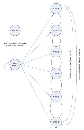
Figure 5: Motor 6-Step States Diagram
