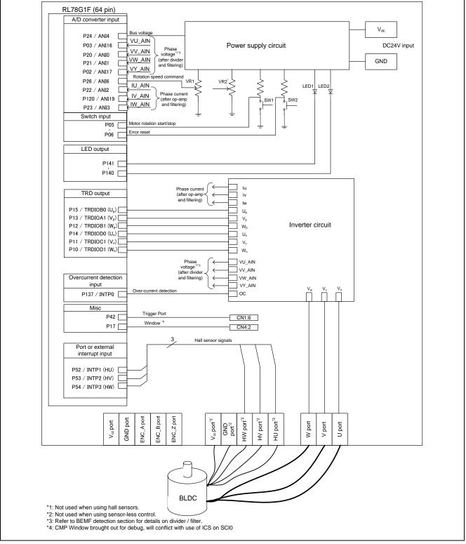
Figure 1: Hardware Configuration Diagram
