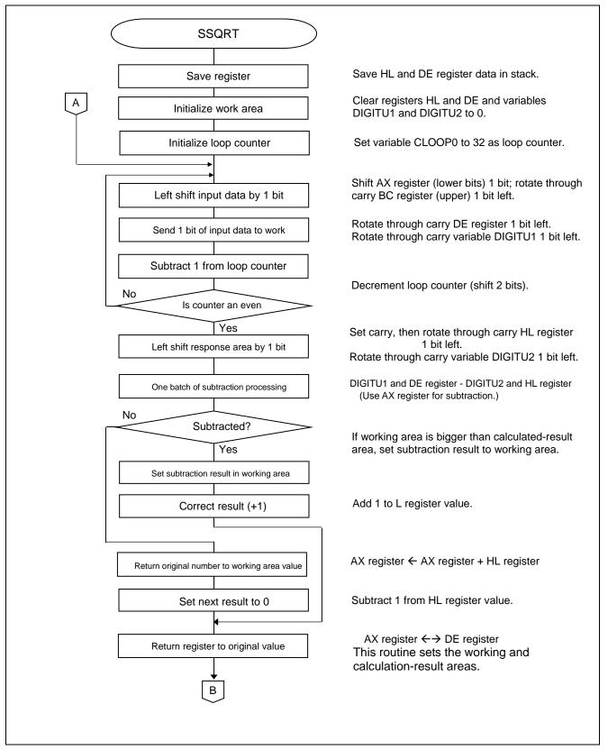
Figure 3.5 Square Root Operation Flowchart (1/2)
