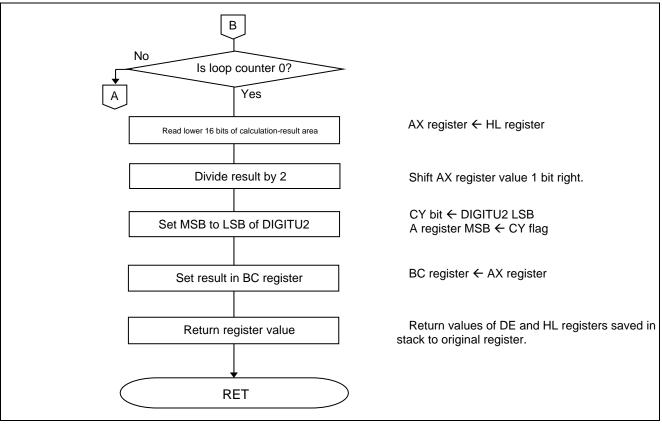
Figure 3.6 Square Root Operation Flowchart (2/2)
