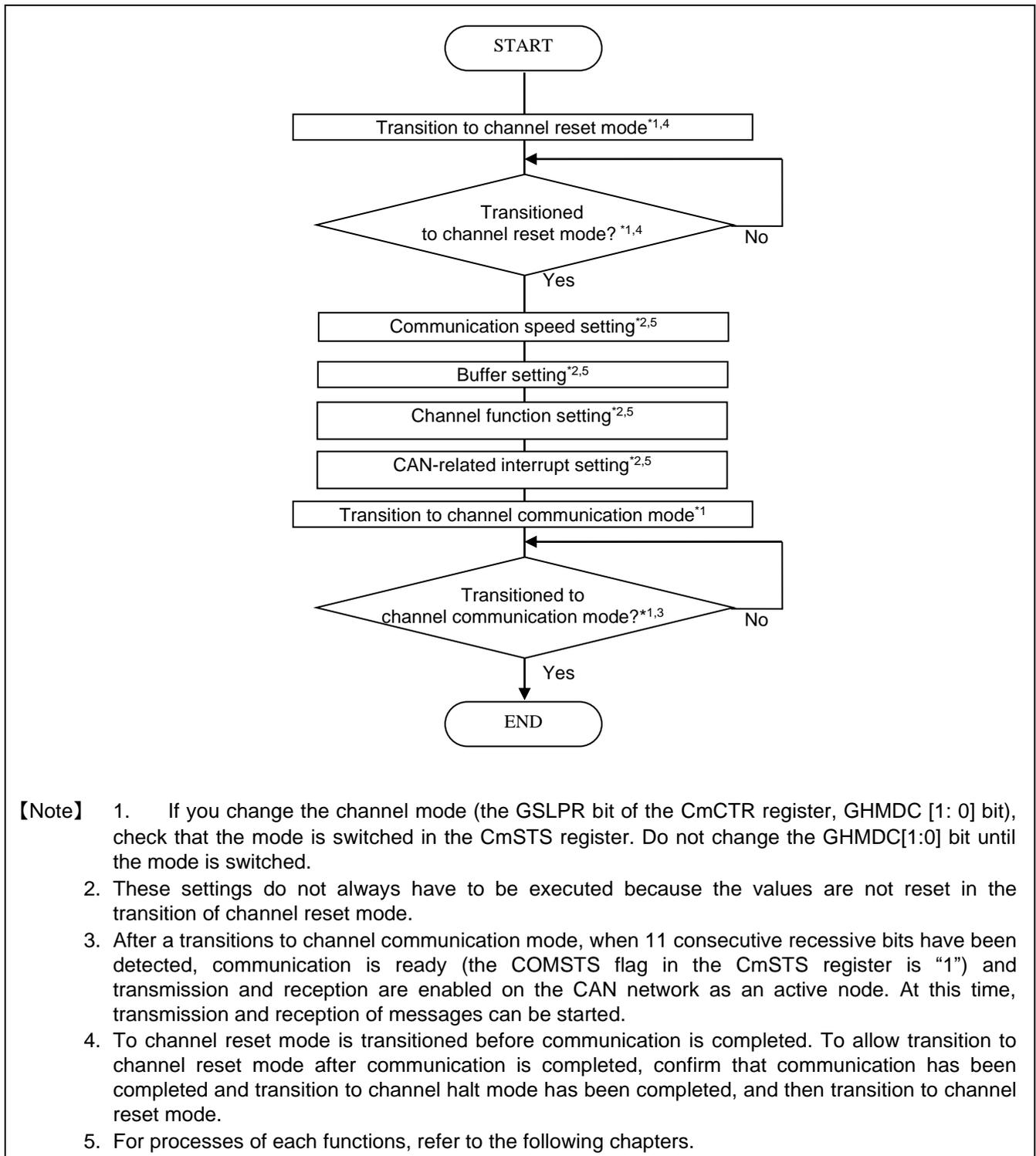
Figure 1-4 Procedure of CAN Configuration after Channel Reset Mode
