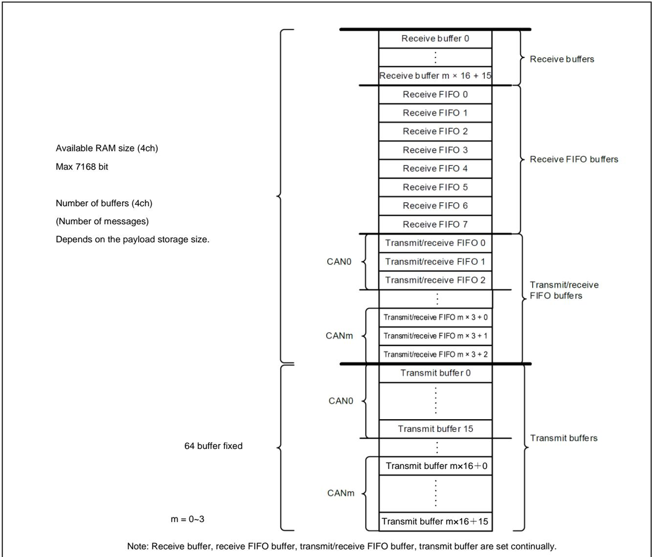
Figure 6-1 Buffer Configuration
