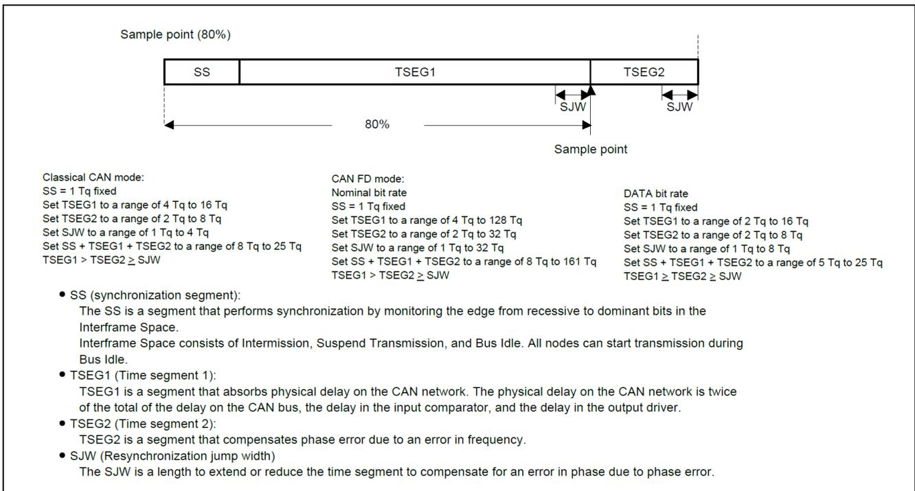
Figure 3-1 Bit Segment Components and Sample Point
