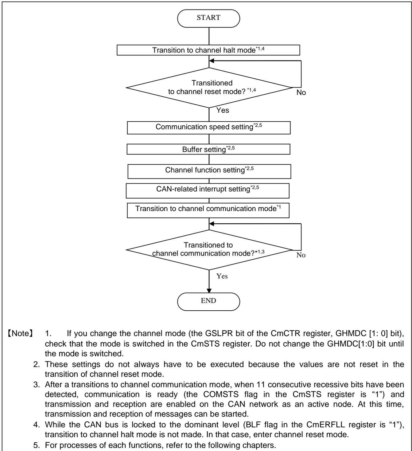
Figure 1-5 Procedure of CAN Configuration after Channel Halt Mode
