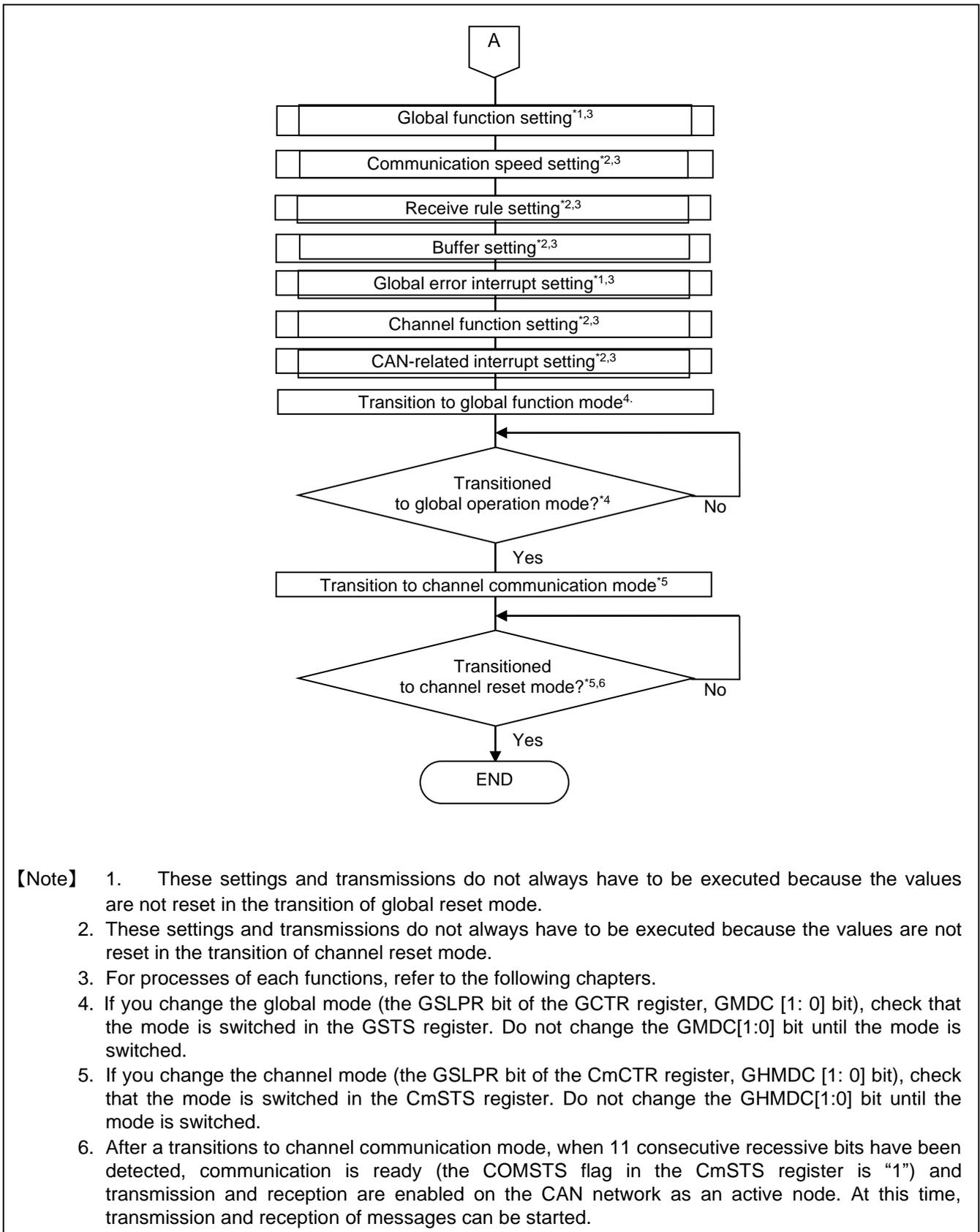
Figure 1-3 Procedure of CAN Configuration after Global Reset Mode 2/2
