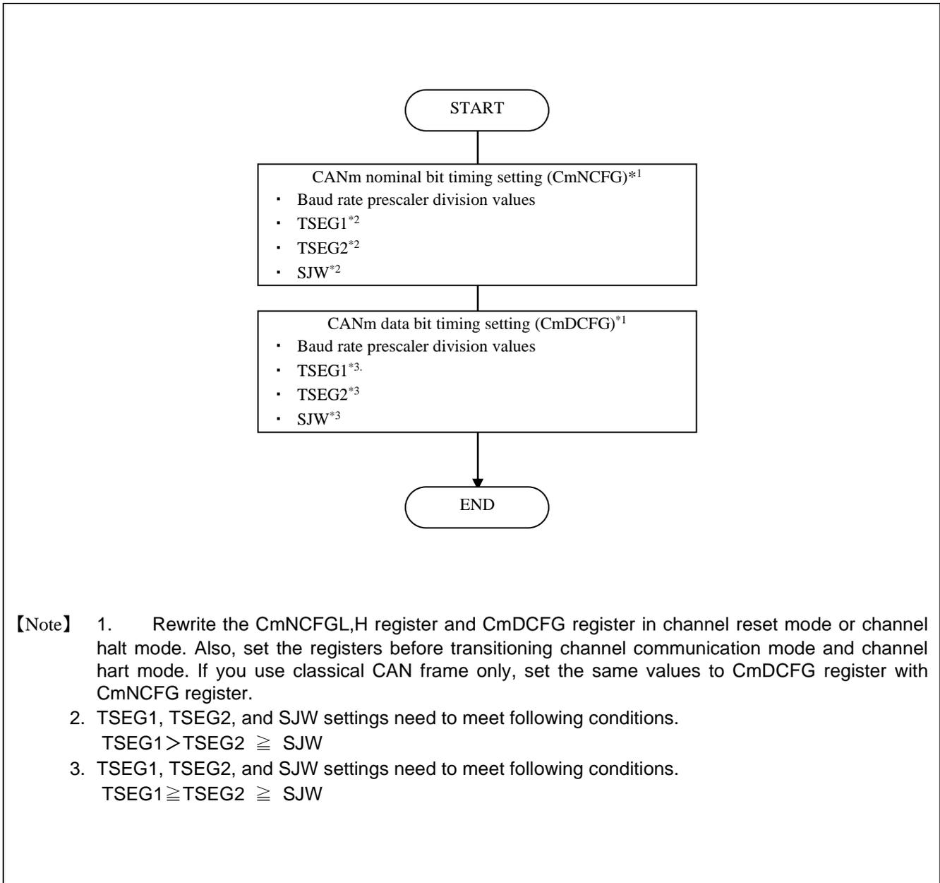
Figure 3-2 5.1 Setting up CAN Bit Timing and Communication Speed
