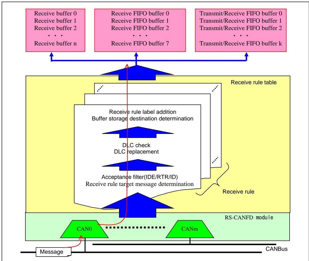
Figure 5-1 Filtering Image by Receive Rule Table
