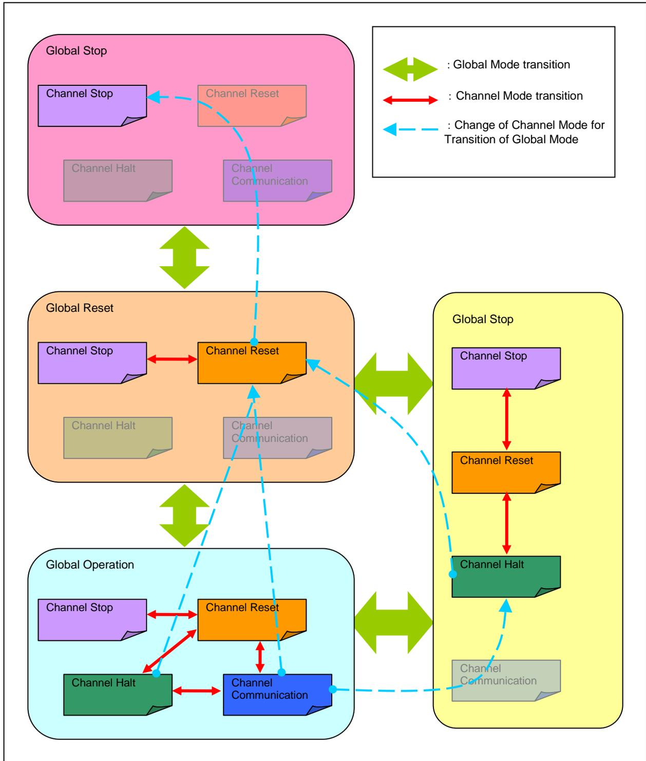
Figure 2-3 Transitions of Global Mode and Channel Mode
