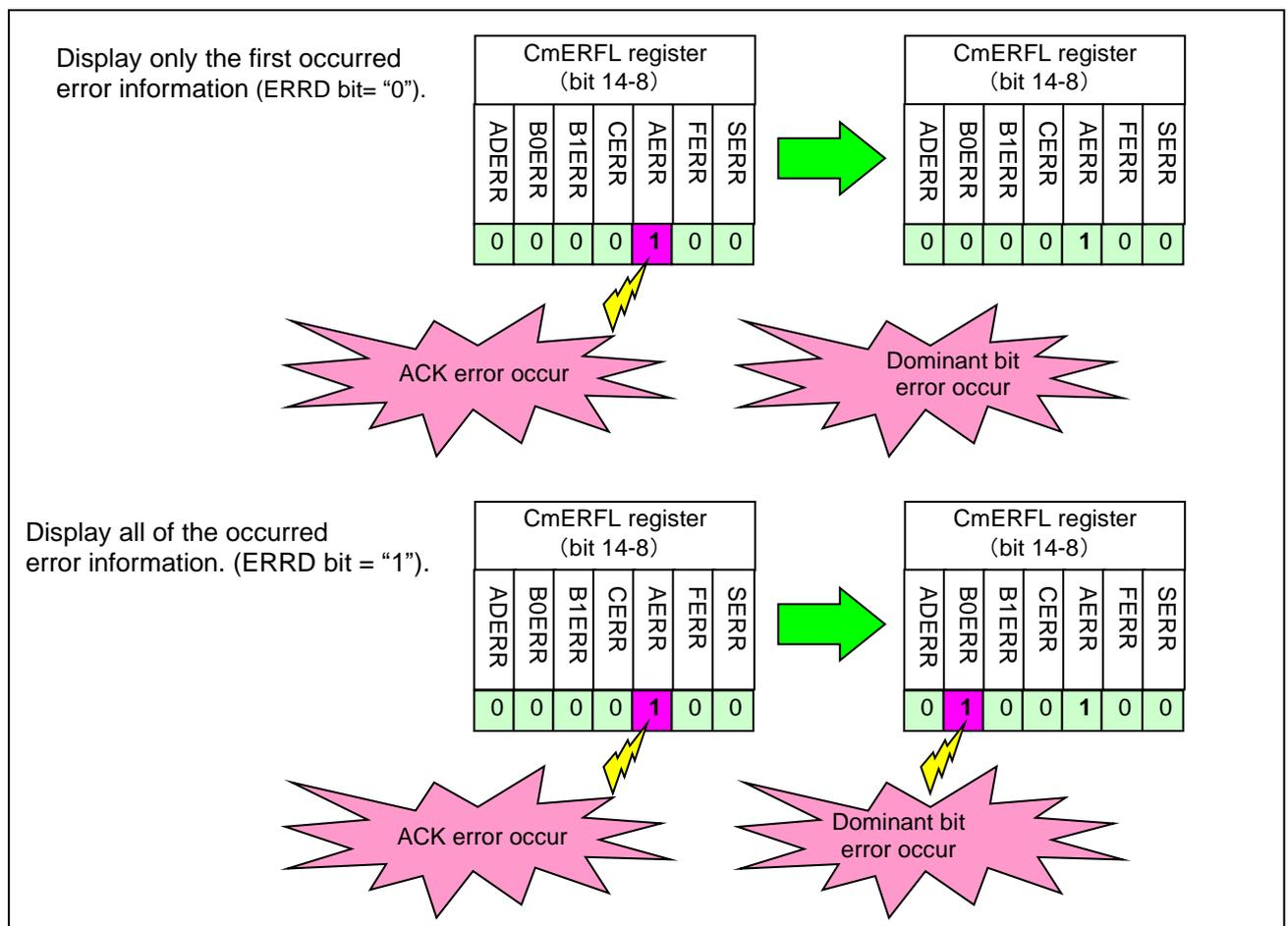
Figure 8-5 Operation Example of Error Display Mode
