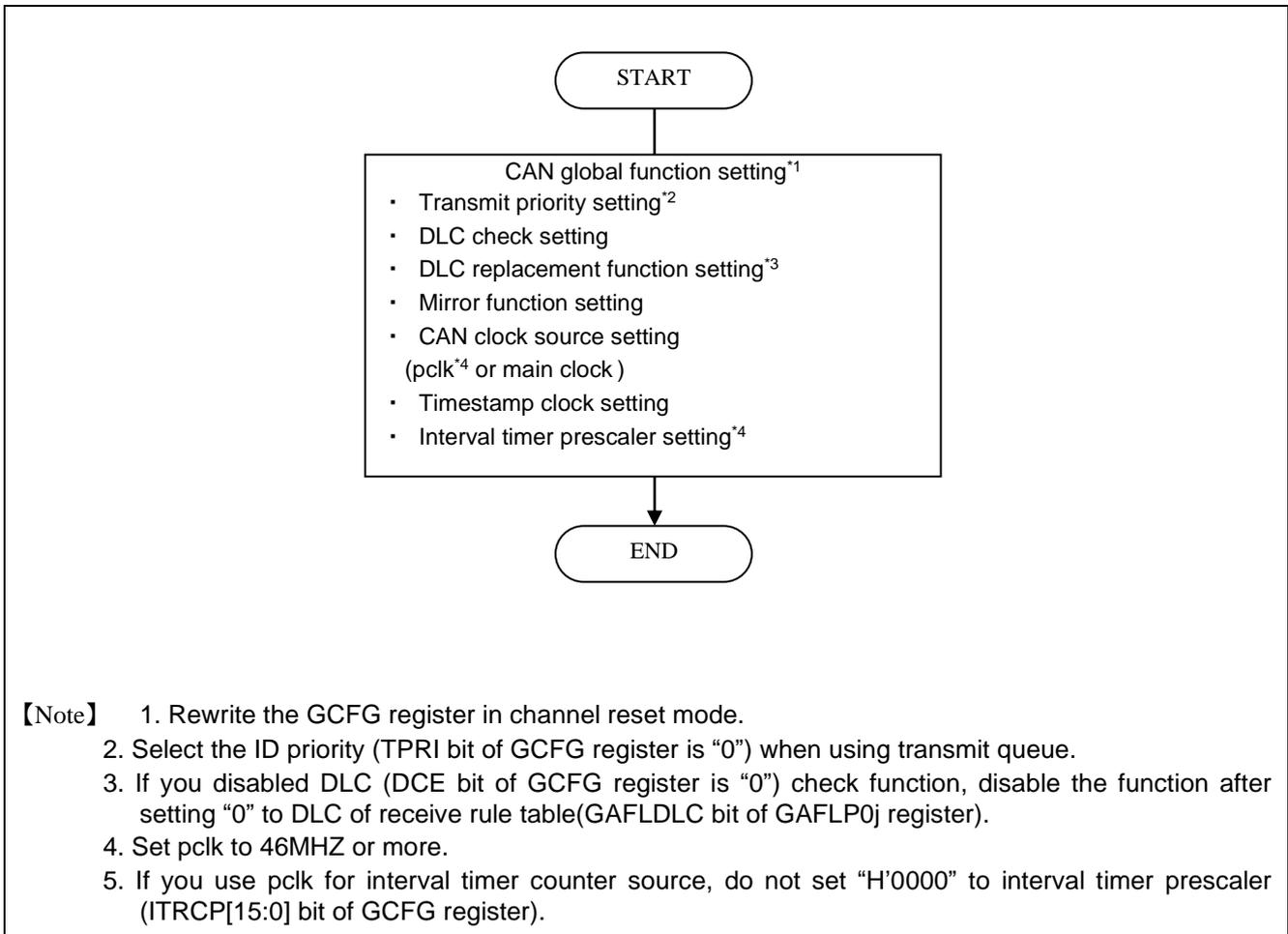
Figure 4-2 Global Function Setting Procedure
