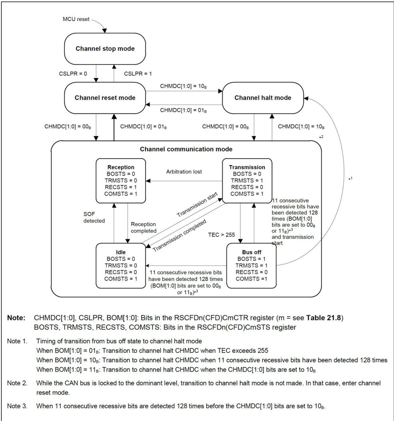
**Note:** CHMDC[1:0], CSLPR, BOM[1:0]: Bits in the RSCFDn(CFD)CmCTR register (m = see Table 21.8)
