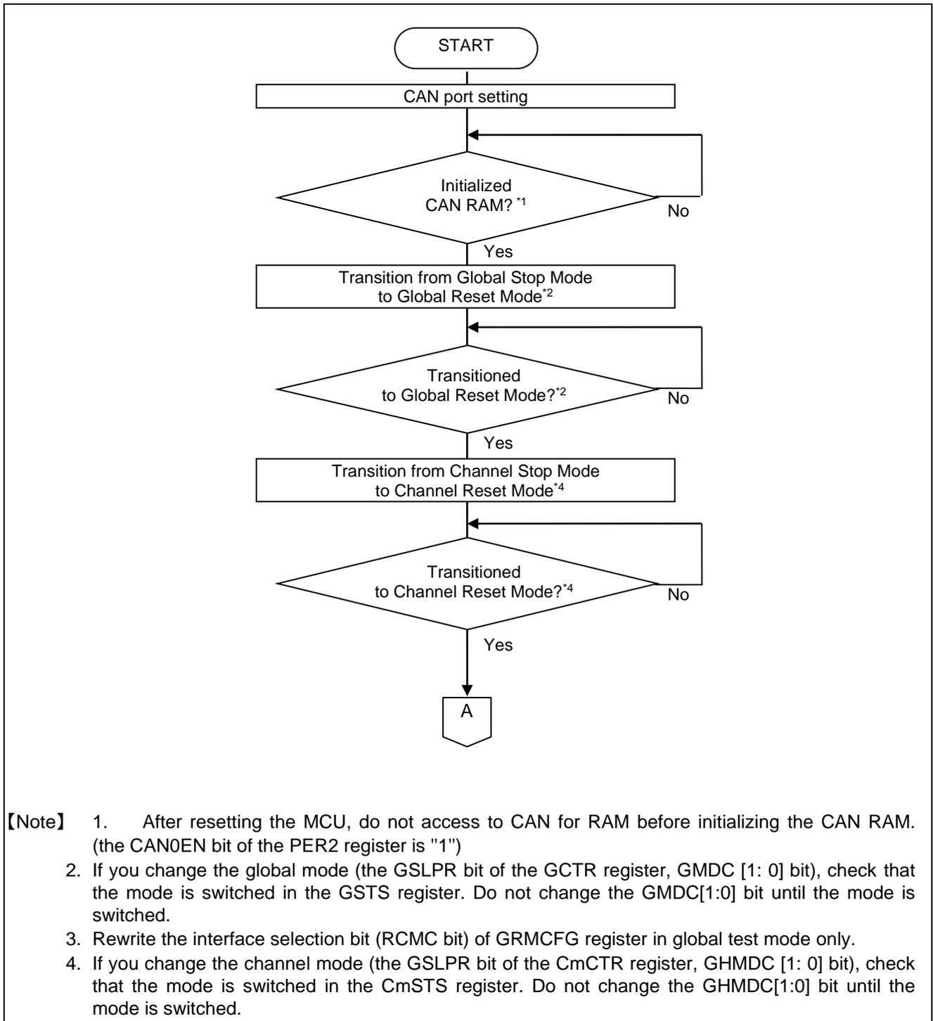
Figure 1-1 Procedure of CAN Configuration after resetting MCU 1/2
