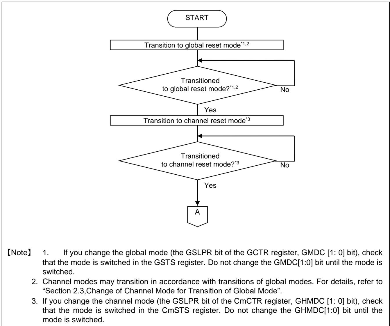
Figure 1-2 Procedure of CAN Configuration after Global Reset Mode 1/2
