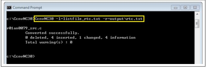
Figure 4.2 CcnvNC30 Execution Window (Clock Operation Using RTC)
