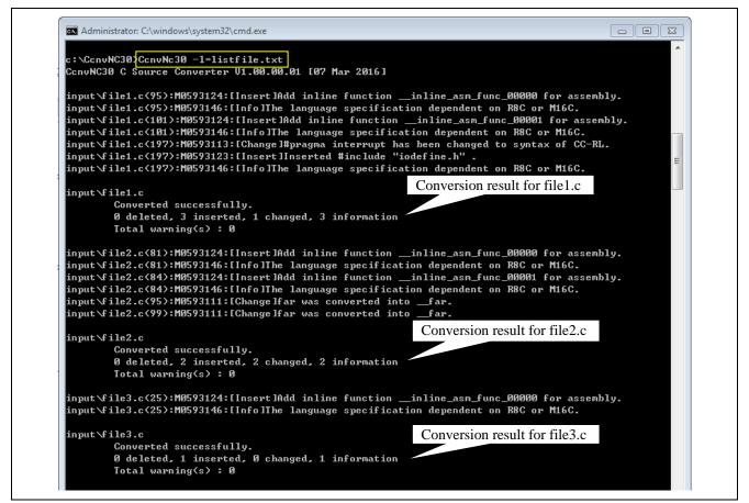
Figure 2.3 CcnvNC30 Execution Window (Multiple Files)
