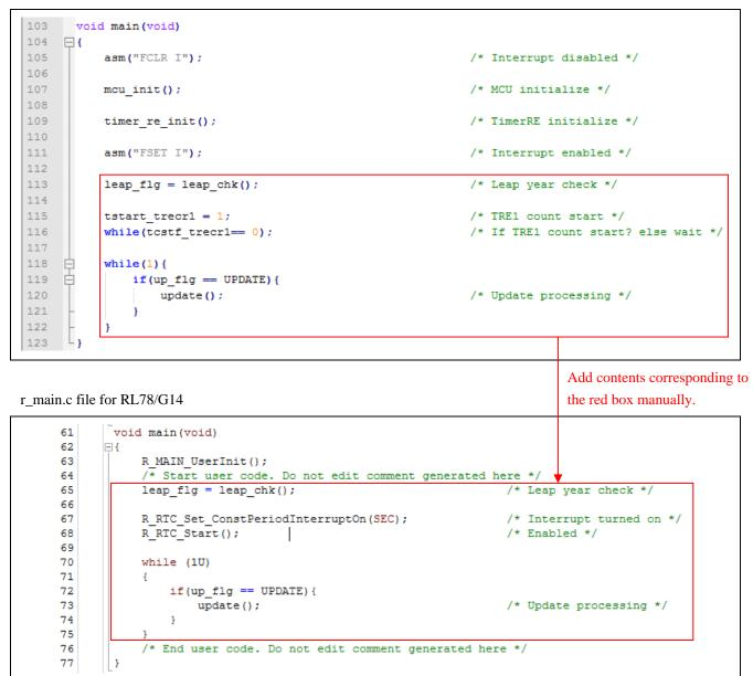
Figure 4.8 Replacement of main Function
