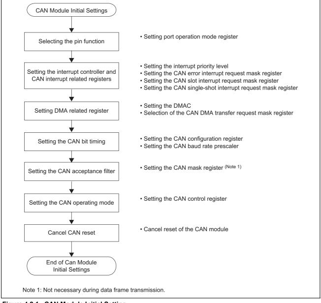
Figure 4.2.1 CAN Module Initial Setting
