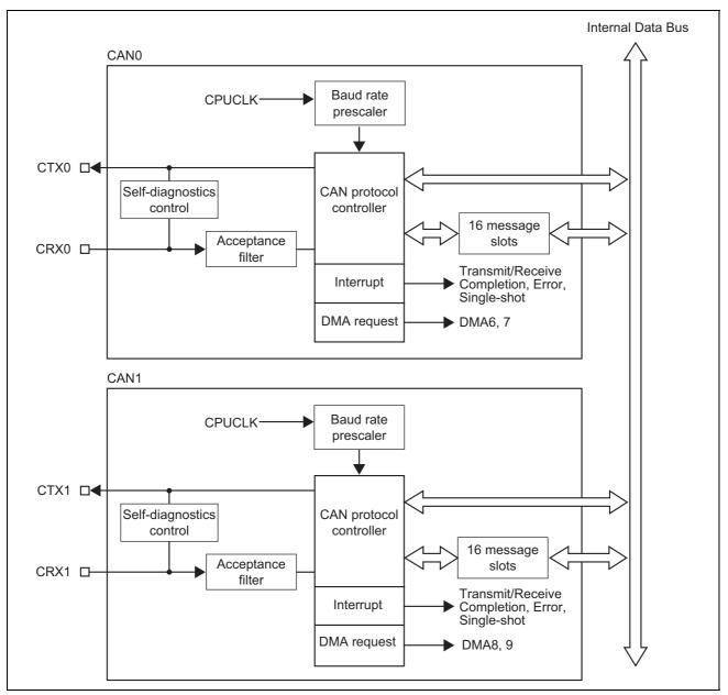
Figure 3.1.1 CAN Module Block Diagram
