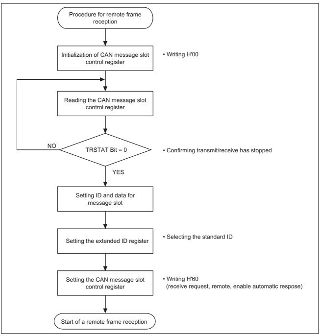
Figure 4.3.1 Remote Frame Reception Processing
