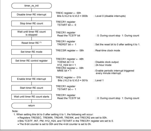
Figure 4.15 Initial Setting of Timer RE
