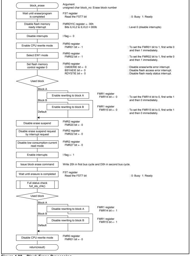
Figure 4.22 Block Erase Processing
