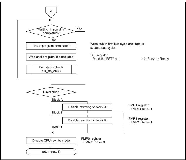
Figure 4.24 Program Command Processing (2/2)
