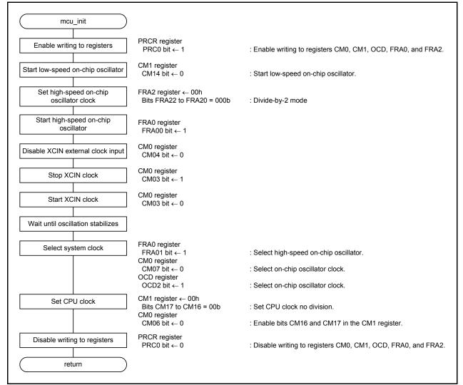
Figure 4.13 System Clock Setting
