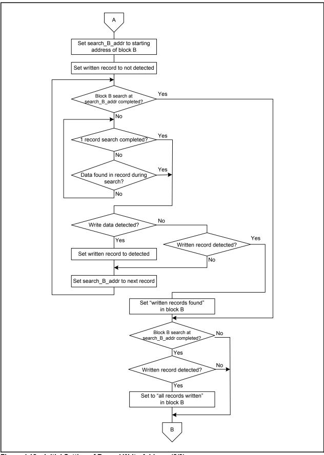
Figure 4.18 Initial Setting of Record Write Address (2/3)
