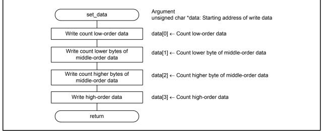
Figure 4.21 Write Data Setting
