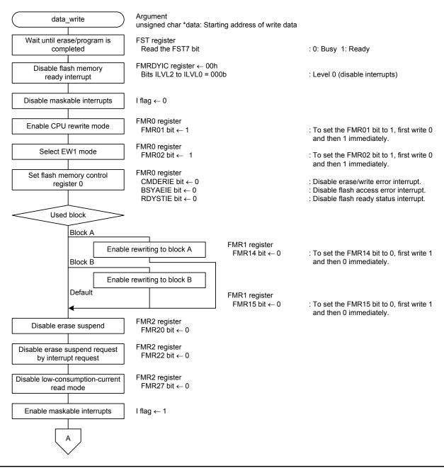
Figure 4.23 Program Command Processing (1/2)
