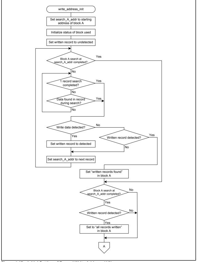
Figure 4.17 Initial Setting of Record Write Address (1/3)
