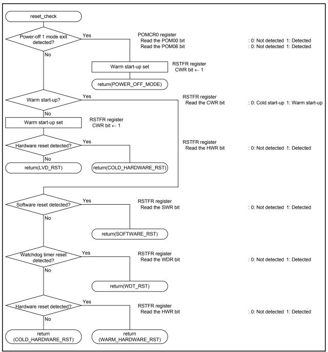
Figure 4.12 Reset Source Determination
