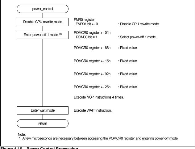
Figure 4.16 Power Control Processing
