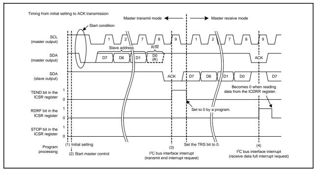
Figure 3.5 Master Receive Timing (1)
