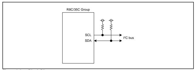
Figure 3.2 Block Diagram
