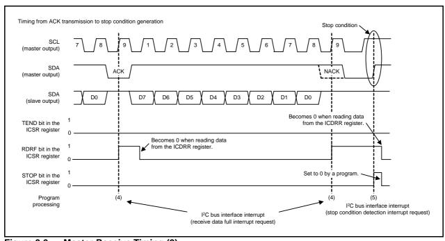
Figure 3.6 Master Receive Timing (2)
