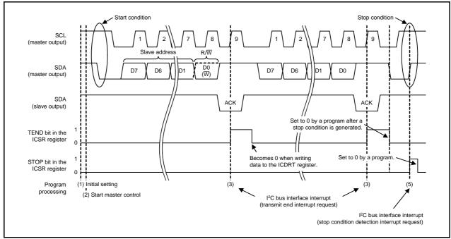
Figure 3.4 Master Transmit Timing
