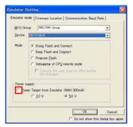
Figure 9 E8a Power Supply Check Box
