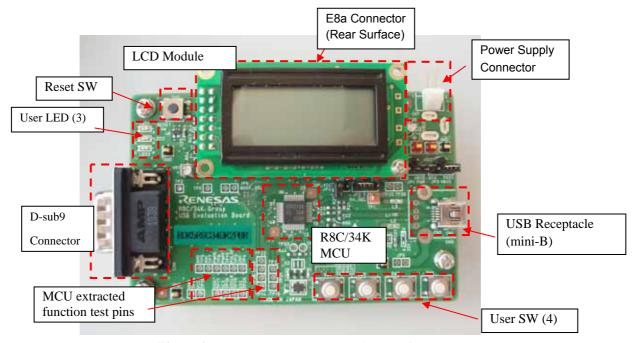
Figure 1 R0K5R8C34DK2PBR Board (Top View)
