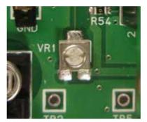
Figure 13 semi-fixed resistor (VR1)
