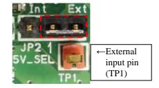
Figure 5 JP2 5V-dedicated power supply switch "Internal input (int)" setting
