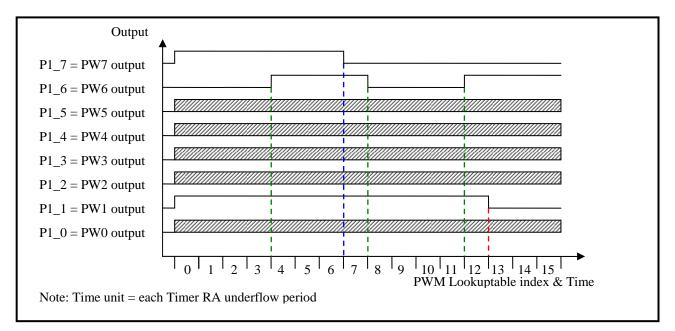
Figure 2 Port output states & PWM Look-up table relationship during DTC transfers
