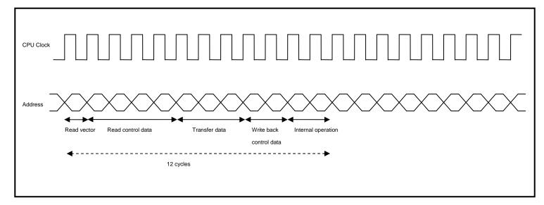
Figure 6 DTC Operation Timing for this application
