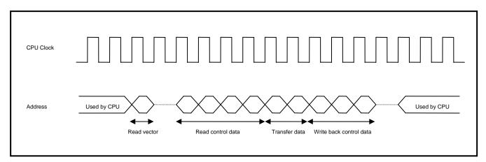
Figure 5 Example of DTC Operation Timing
