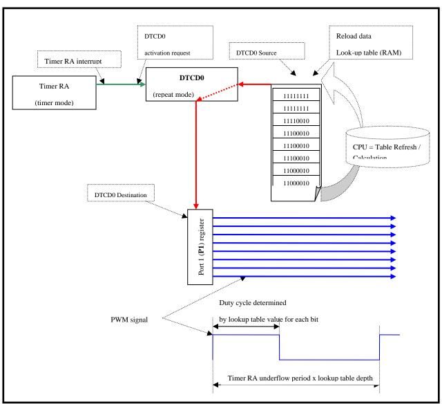
Figure 1 Operation Block Diagram
