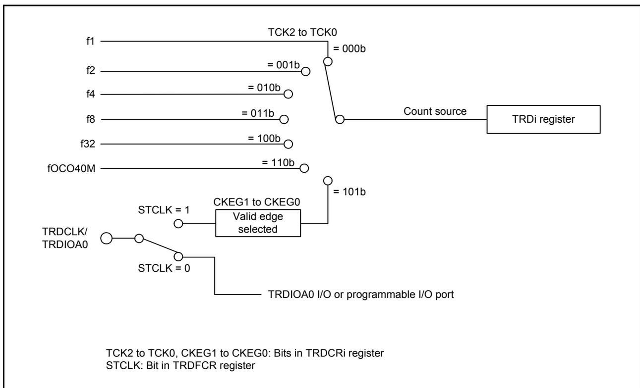
Figure 3.2 Block Diagram of Count Source
