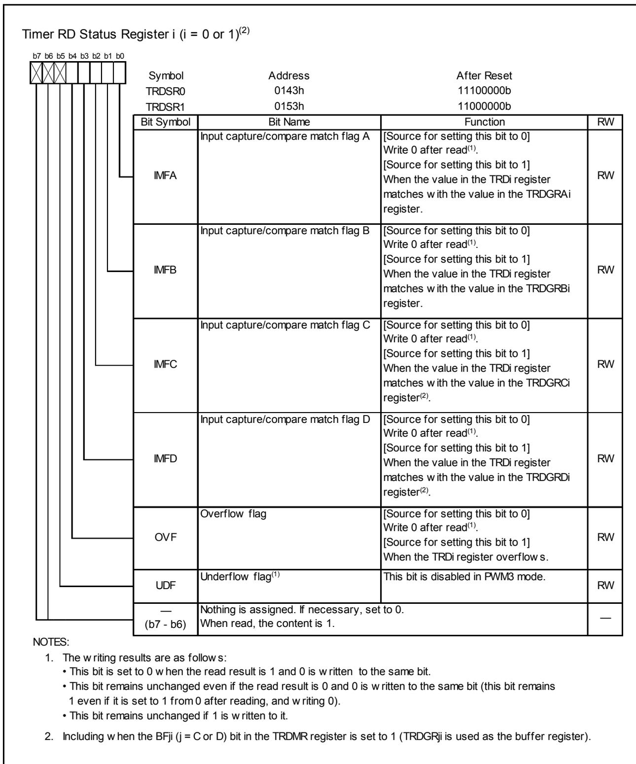
Figure 3.9 TRDSR0 Register in PWM3 Mode
