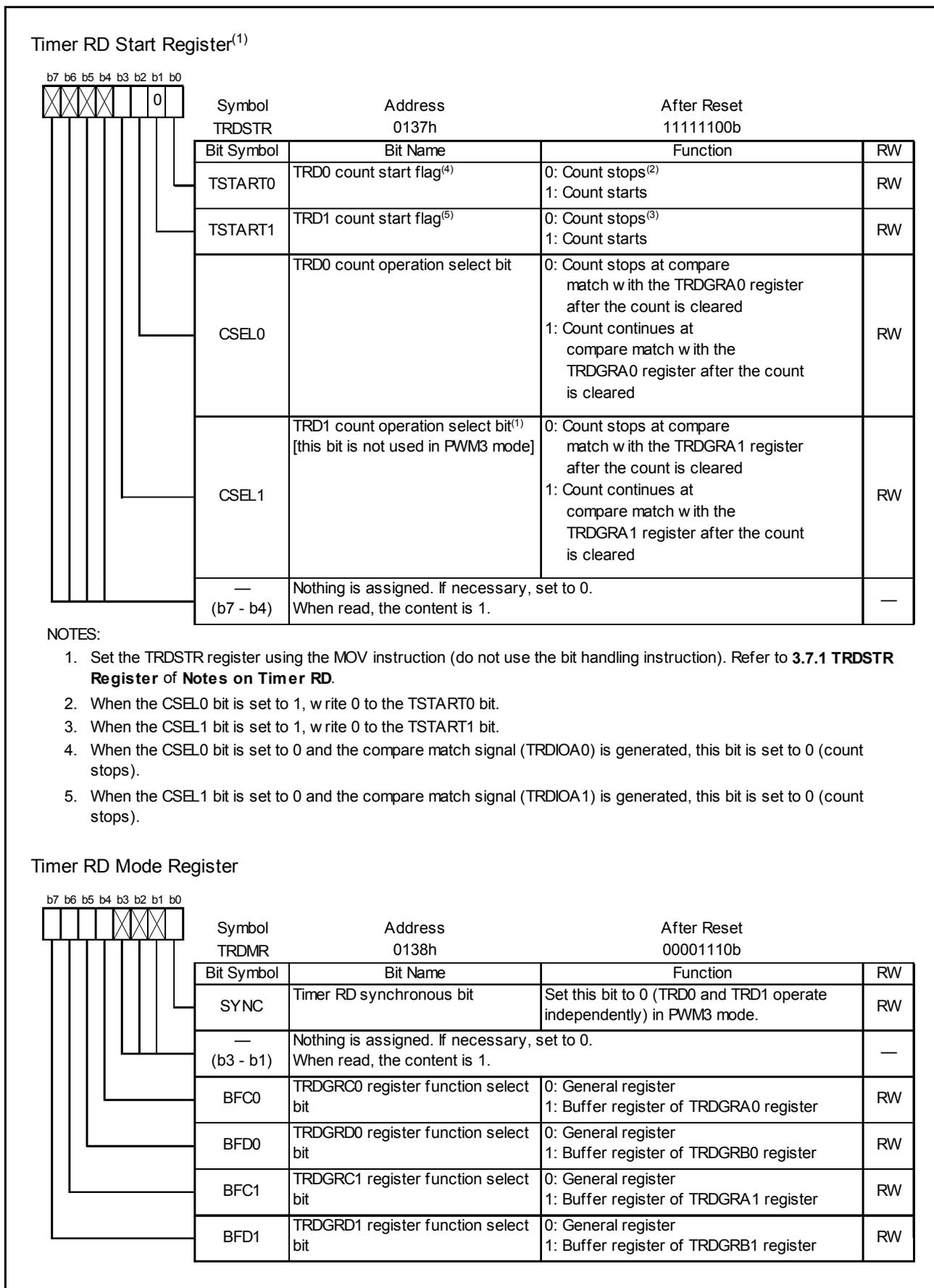
Figure 3.5 Registers TRDSTR and TRDMR in PWM3 Mode
