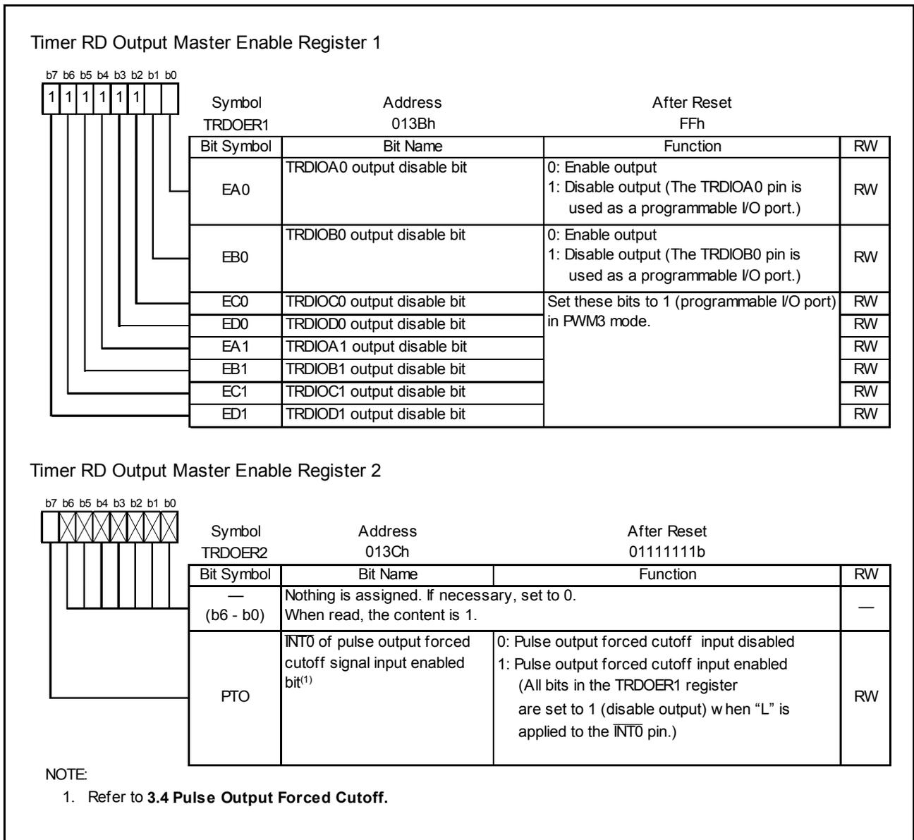
Figure 3.7 Registers TRDOER1 to TRDOER2 in PWM3 Mode
