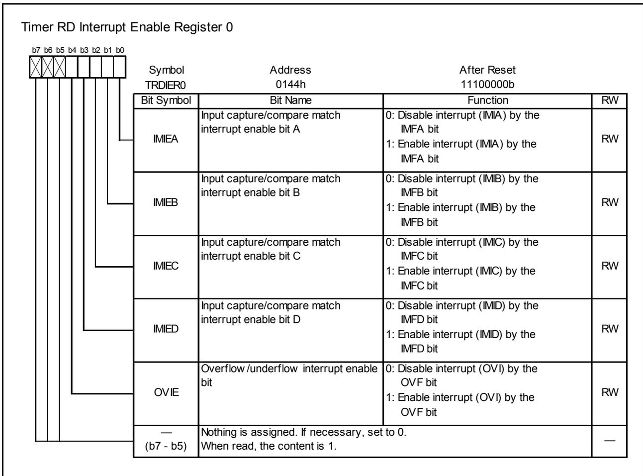
Figure 3.10 TRDIER0 Register in PWM3 Mode
