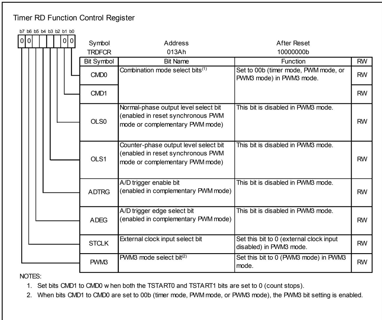
Figure 3.6 TRDFCR Register in PWM3 Mode
