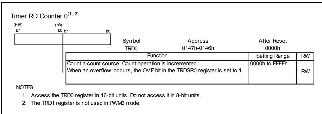
Figure 3.11 TRD0 Register in PWM3 Mode
