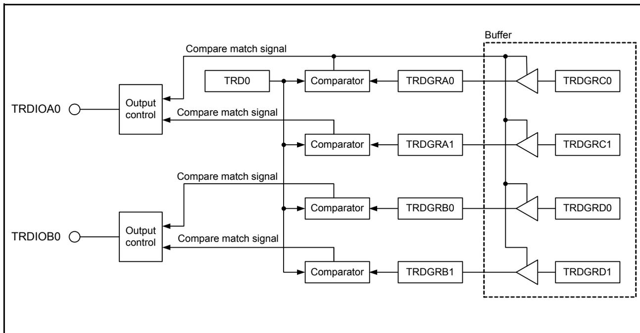
Figure 3.4 Block Diagram of PWM3 Mode
