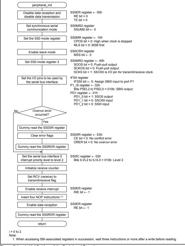
Figure 7.4 Initial Setting of the Peripheral Functions
