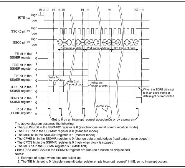
Figure 5.1 shows the Master Transmission Timing Diagram.
