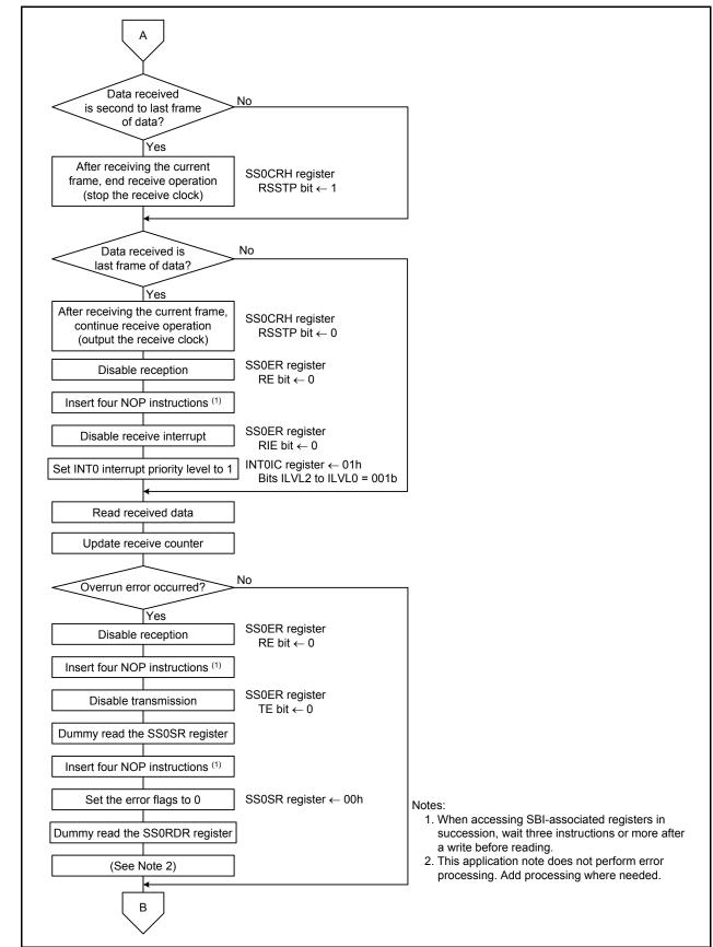
Figure 5.6 Serial Bus Interface 0 Interrupt Handling (2/2)
