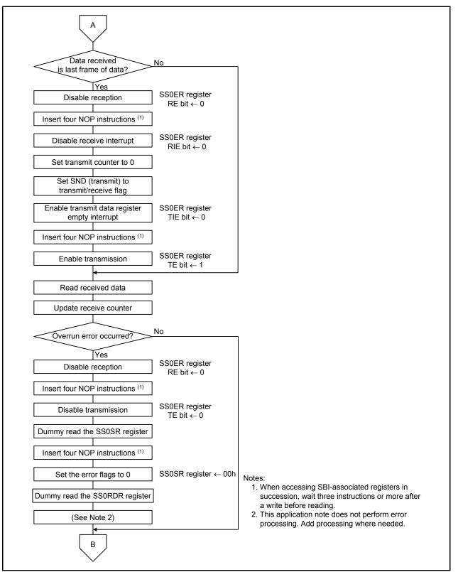
Figure 7.6 Serial Bus Interface 0 Interrupt Handling (2/2)
