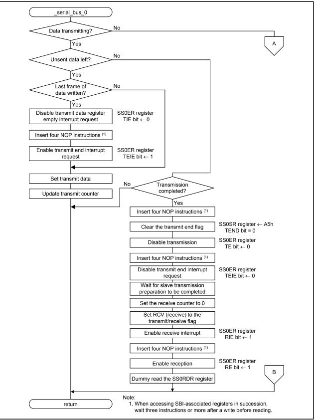
Figure 5.5 Serial Bus Interface 0 Interrupt Handling (1/2)
