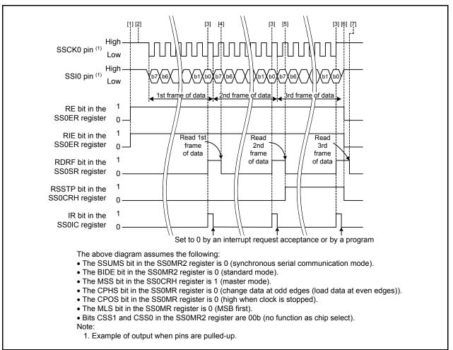
Figure 5.2 Master Reception Timing Diagram
