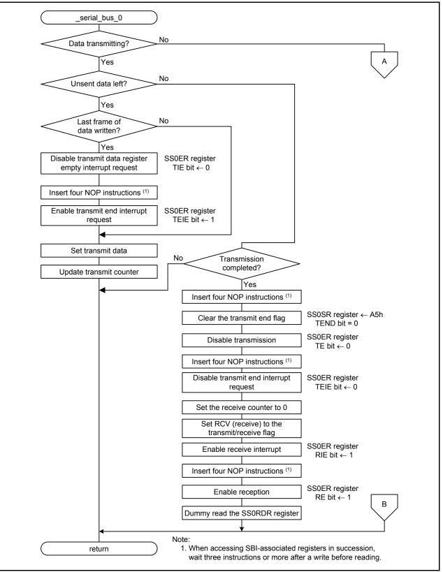
Figure 7.5 Serial Bus Interface 0 Interrupt Handling (1/2)
