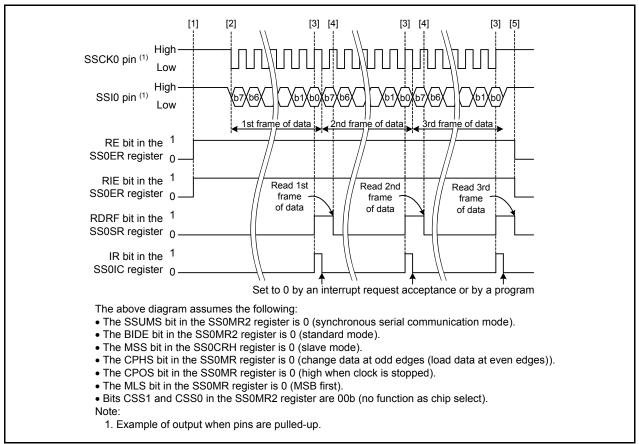
Figure 7.1 shows the Slave Reception Timing Diagram.
