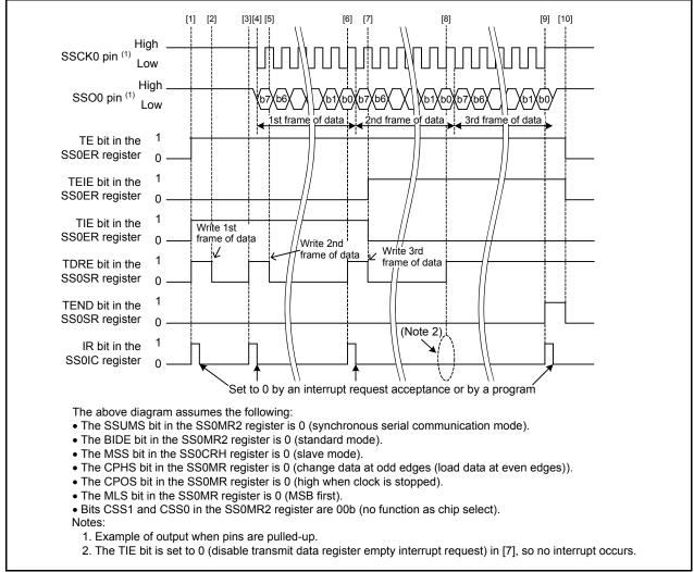
Figure 7.2 shows the Slave Transmission Timing Diagram.
