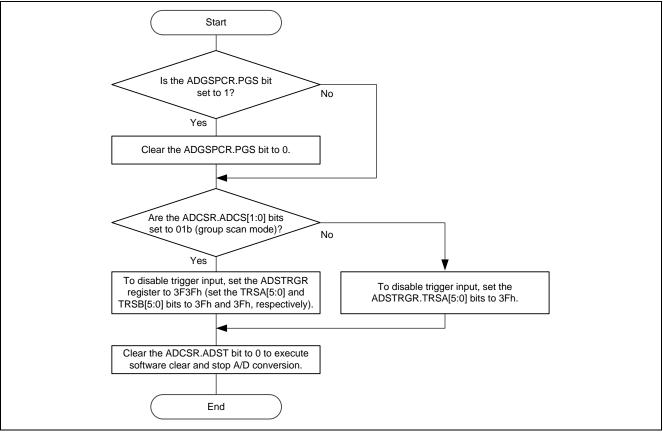
Figure 4.1 Setting Flowchart of Software Clearing Using ADCSR.ADST Bit
