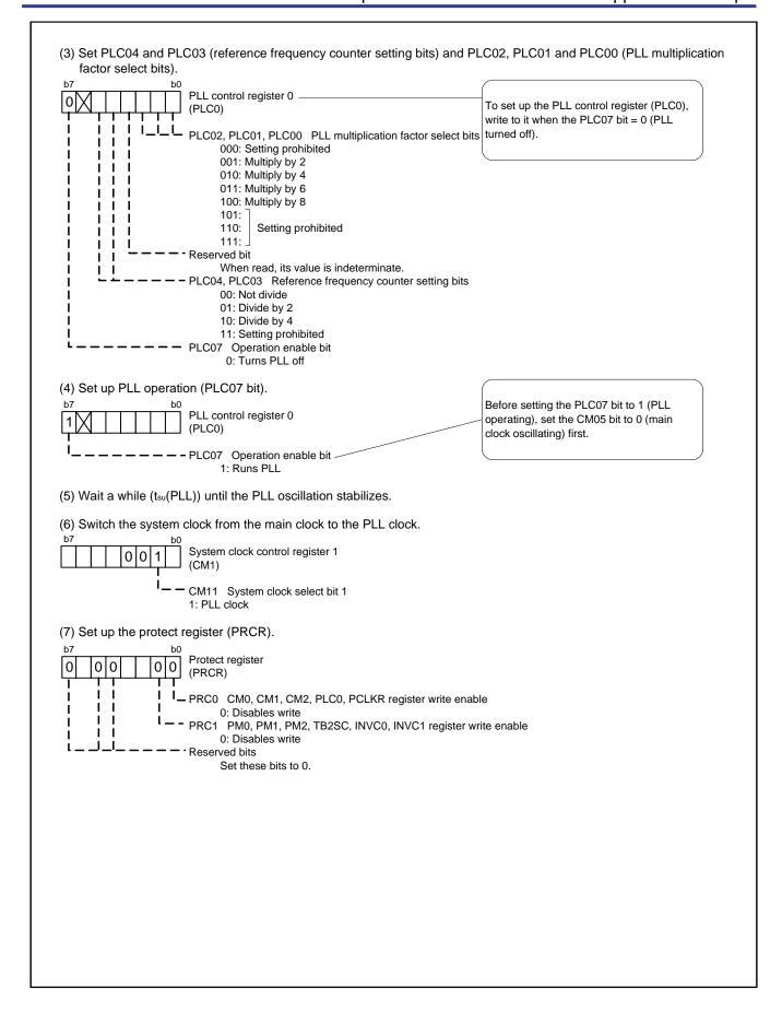
Figure 5. Procedure for Setting Up the Registers to Use the Oscillation Stop/Reoscillation Detect Function (2)
