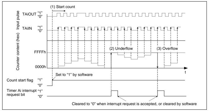
Figure 1. Operation Timing of 2-Phase Pulse Signal Process in Event Counter Mode, Normal Mode
