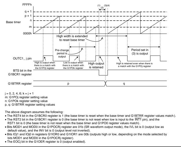
Figure 3.3 Output When Changing the Period After the Base Timer and G1POj Register Values Match and Before the Base Timer and G1POk Register Values Match
