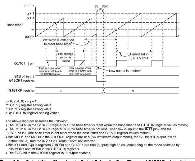
Figure 3.2 Output When Changing the Period Before the Base Timer and G1POj Register Values Match
