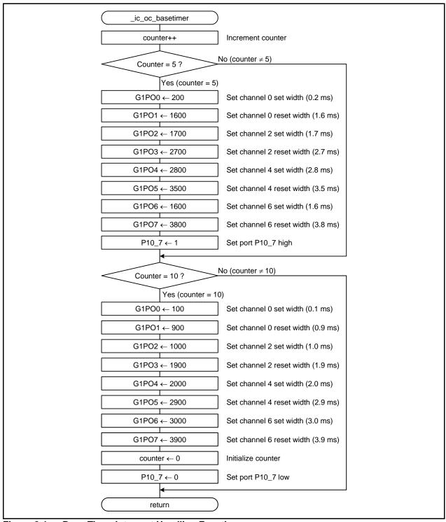
Figure 2.4 Base Timer Interrupt Handling Function
