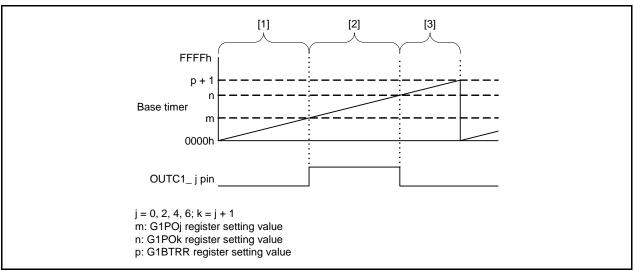
Figure 3.1 Timing Diagram for Period Change When Using SR Waveform Output Mode
