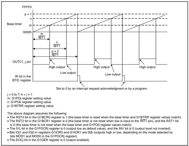
Figure 1.1 SR Waveform Output Mode Operation
