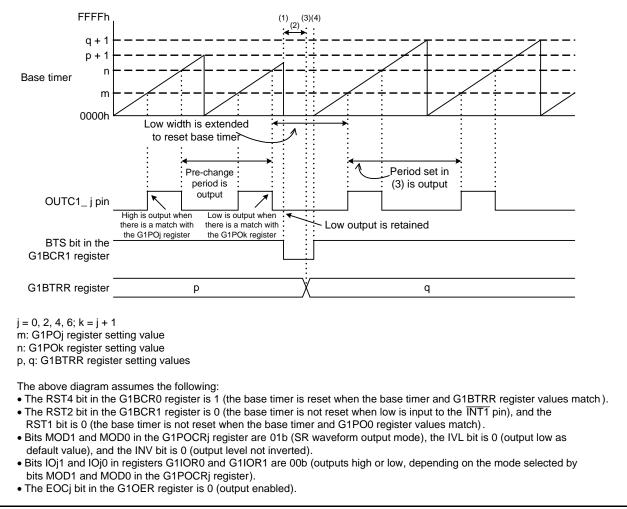
Figure 3.4 Output When Changing the Period After the Base Timer and G1POk Register Values Match and Before the Base Timer and G1BTRR Register Values Match
