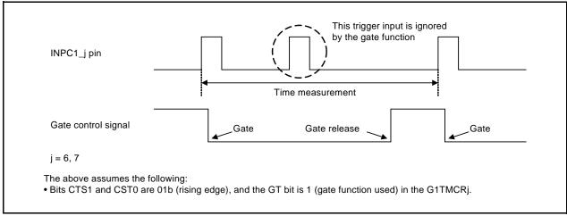
Figure 3.1 Time Measurement Period with Gate Function
