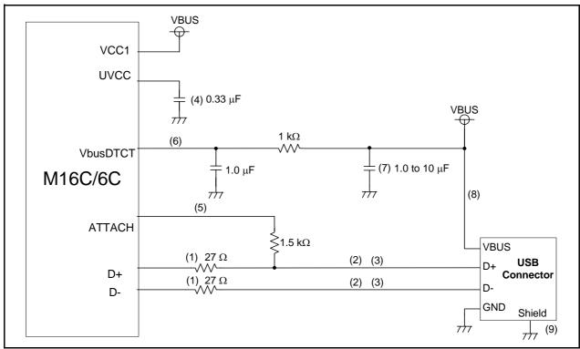
Figure 6.1 Bus-powered Mode Circuit (5.0 V)
