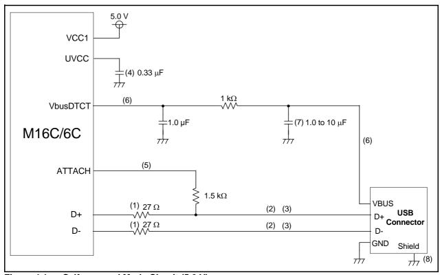
Figure 4.1 Self-powered Mode Circuit (5.0 V)
