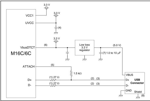
Figure 5.1 Bus-powered Mode Circuit (3.3 V)
