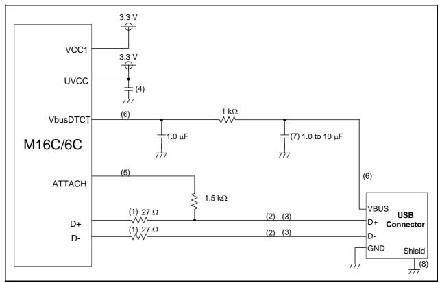
Figure 3.1 Self-powered Mode Circuit (3.3 V)
