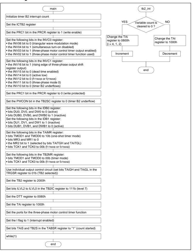
Figure 4. Triangular Wave Modulation (Three-phase Mode 0) Flowchart
