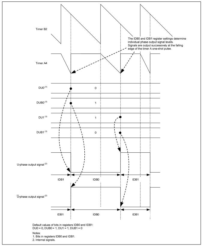
Figure 3. U-phase Output Signal Operation Example
