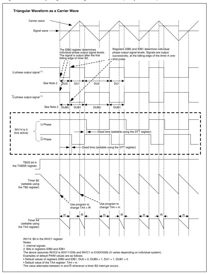
Figure 1. Triangular Wave Modulation (Three-phase Mode 0) Operation
