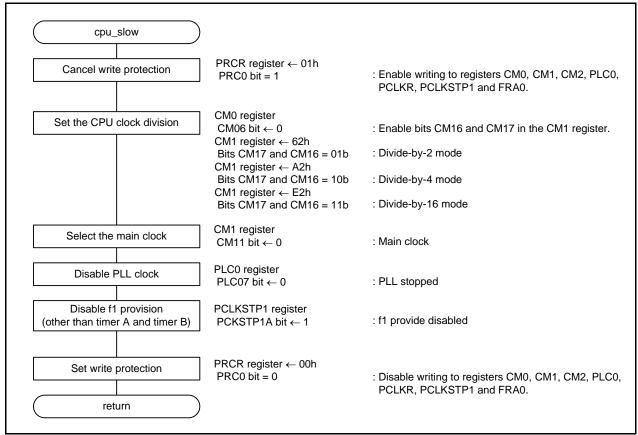
Figure 5.4 CPU Clock Medium-Speed Mode Transition
