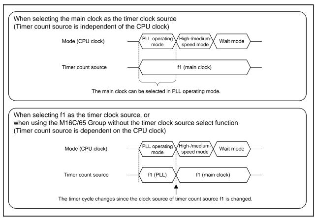
Figure 1.1 Dependence Between the CPU Clock and Timer Count Source
