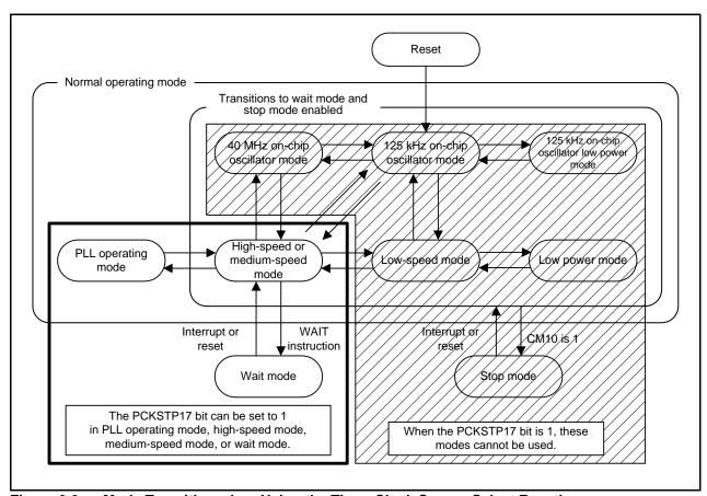
Figure 3.2 Mode Transition when Using the Timer Clock Source Select Function
