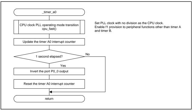
Figure 5.6 Timer A0 Interrupt Handling
