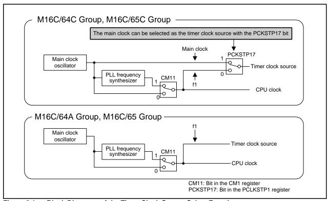
Figure 3.1 Block Diagrams of the Timer Clock Source Select Function
