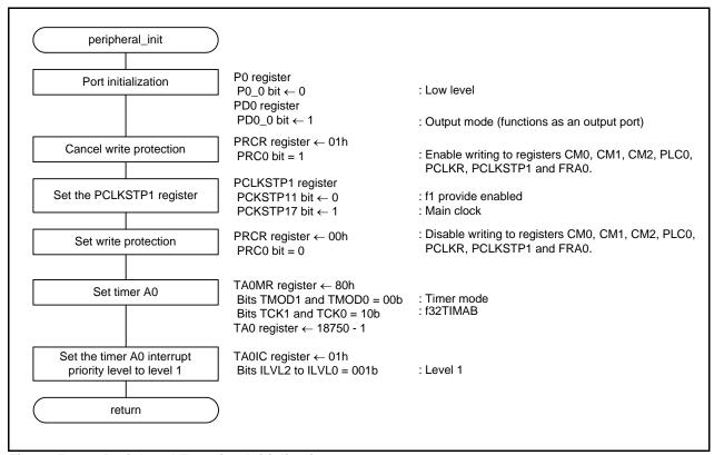
Figure 5.3 Peripheral Function Initialization
