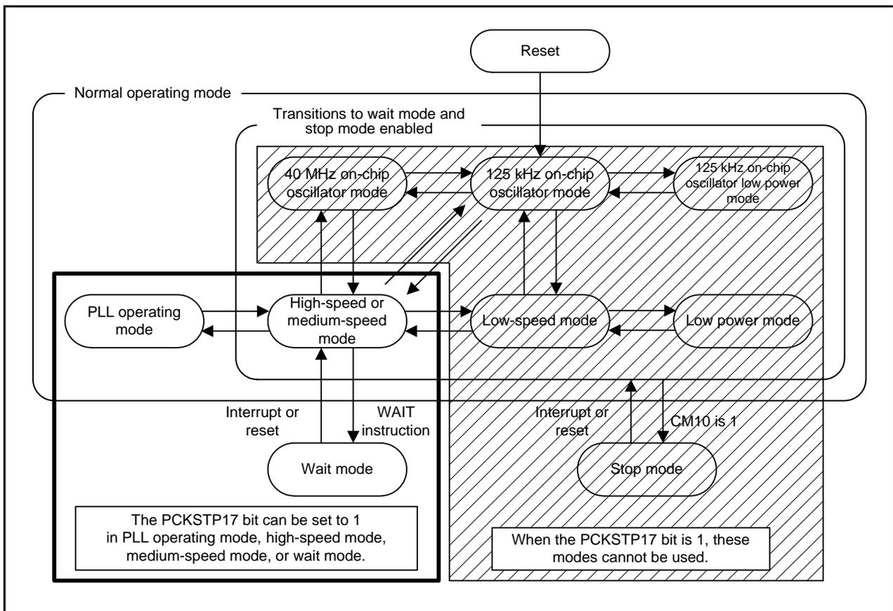
Figure 3.2 Mode Transition when Using the Timer Clock Source Select Function
