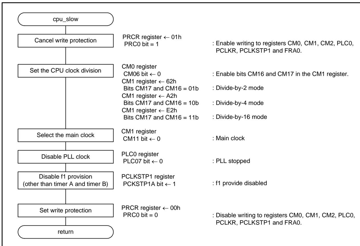
Figure 5.4 CPU Clock Medium-Speed Mode Transition
