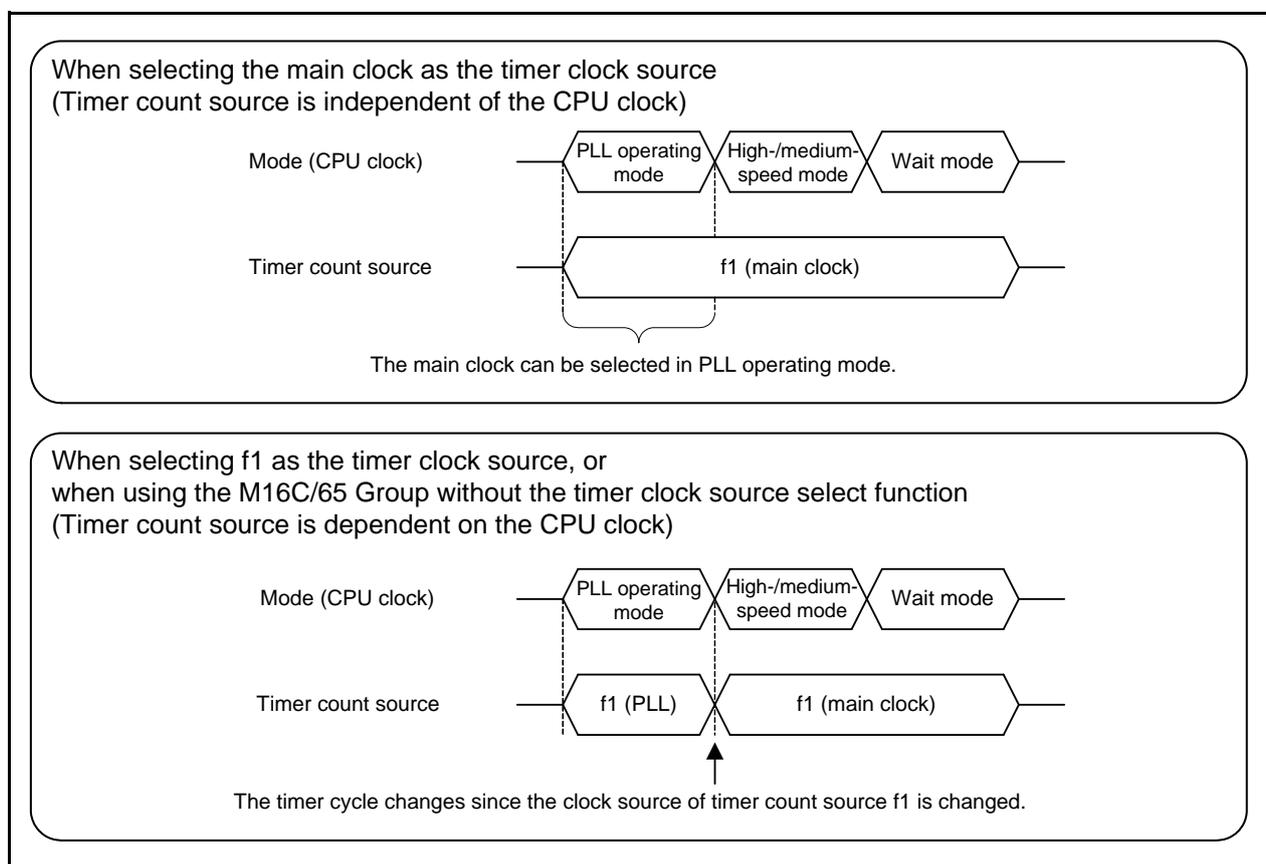
**Figure 1.1 Dependence Between the CPU Clock and Timer Count Source**
