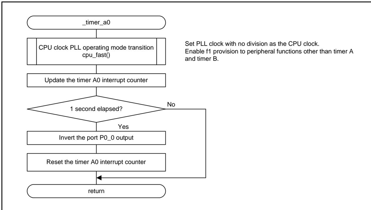
Figure 5.6 Timer A0 Interrupt Handling
