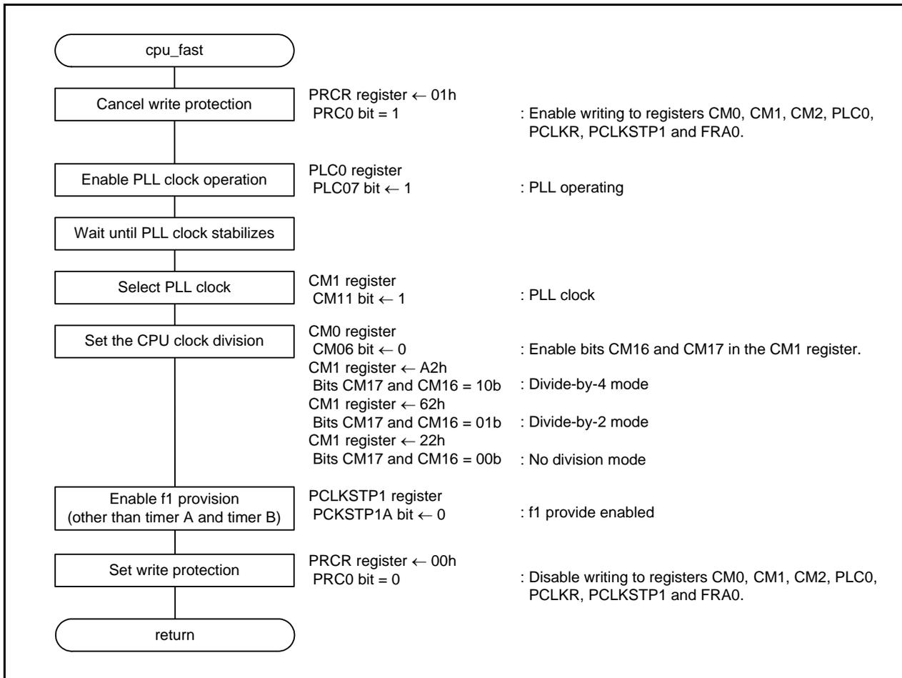
Figure 5.5 CPU Clock PLL Operating Mode Transition
