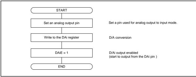
Figure 4.1 D/A Output Operation Procedure (i = 0, 1)
