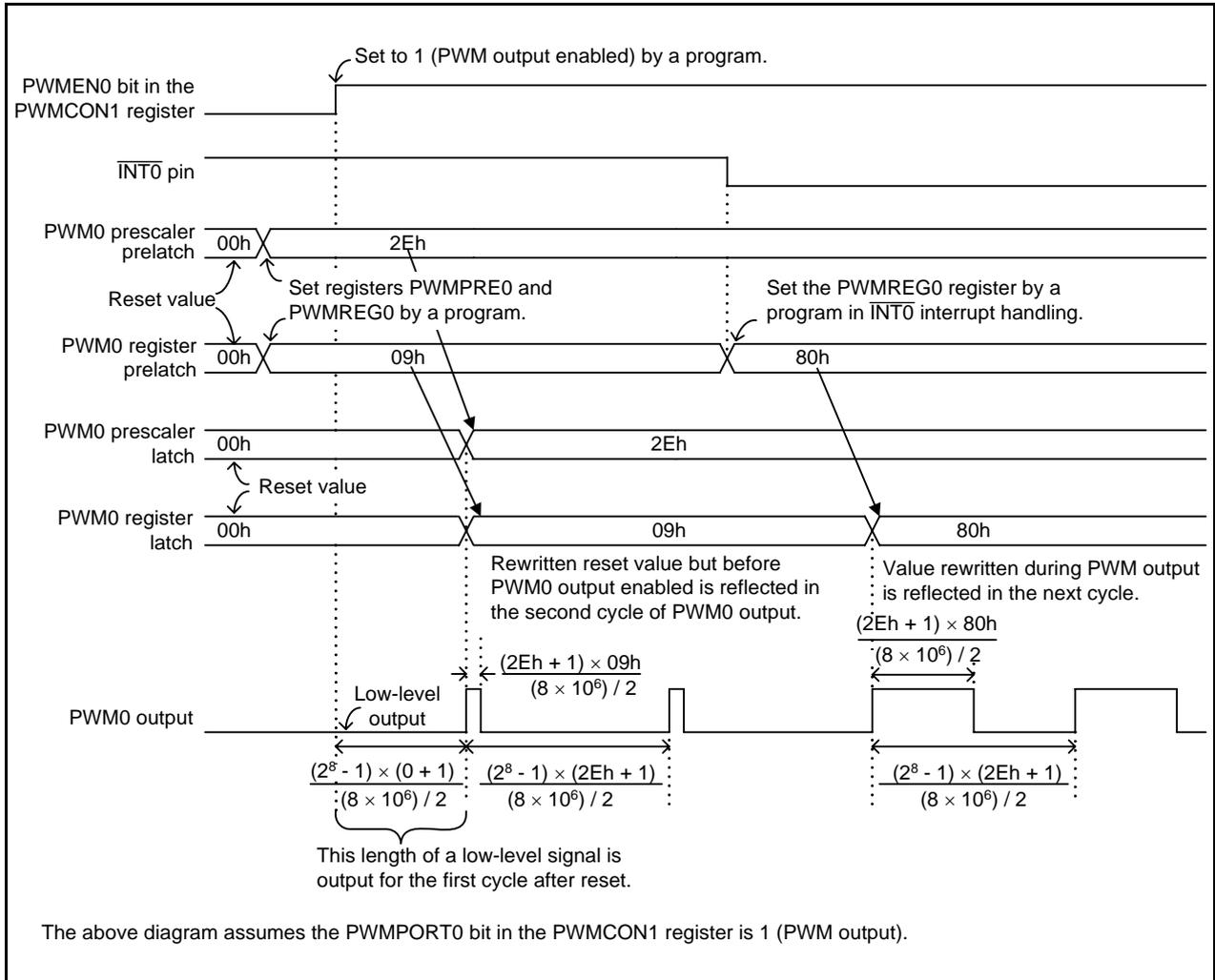
Figure 3.4 PWM0 Output Example of the Sample Program
