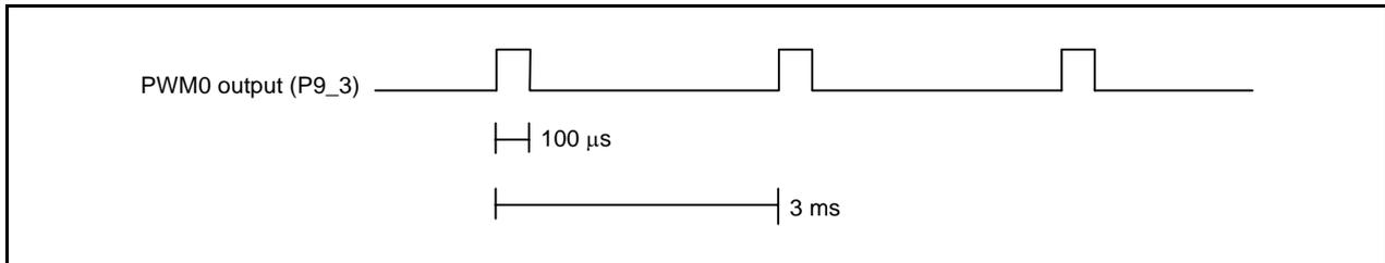
**Figure 3.1 Sample Output Waveform**
