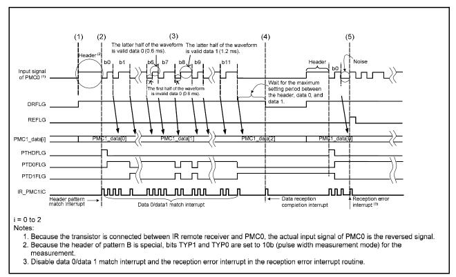
Figure 5.2 PMC1 Reception Timing of the Remote Control with Header and Repeat Code Format
