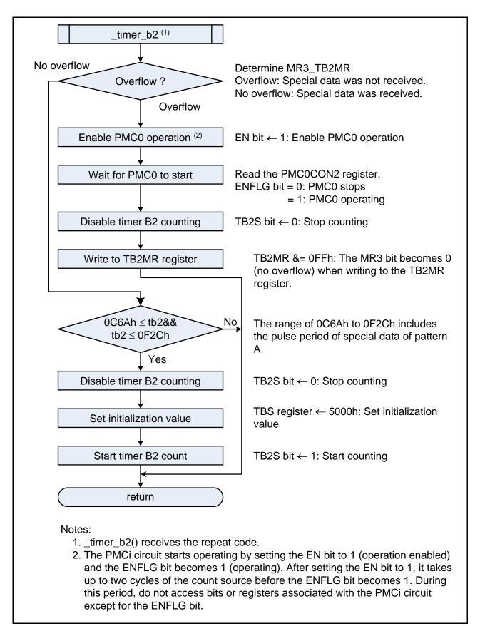
Figure 5.9 Timer B2 Interrupt Handling
