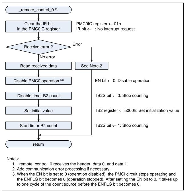
Figure 5.8 PMC0 Interrupt Handling
