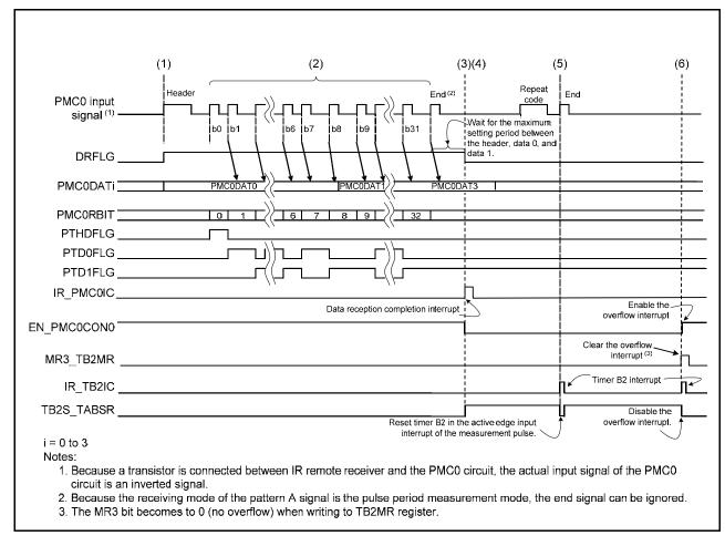
Figure 5.1 shows the status operation and interrupt generation timing of the PMC0 circuit remote control signal during reception.
