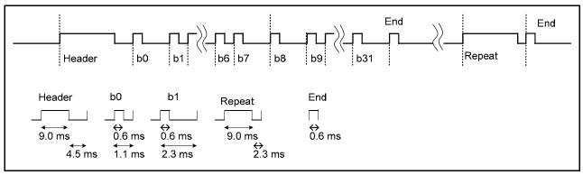
Figure 1.1 Pattern A: Remote Control Format with Header Pattern and Repeat Code
