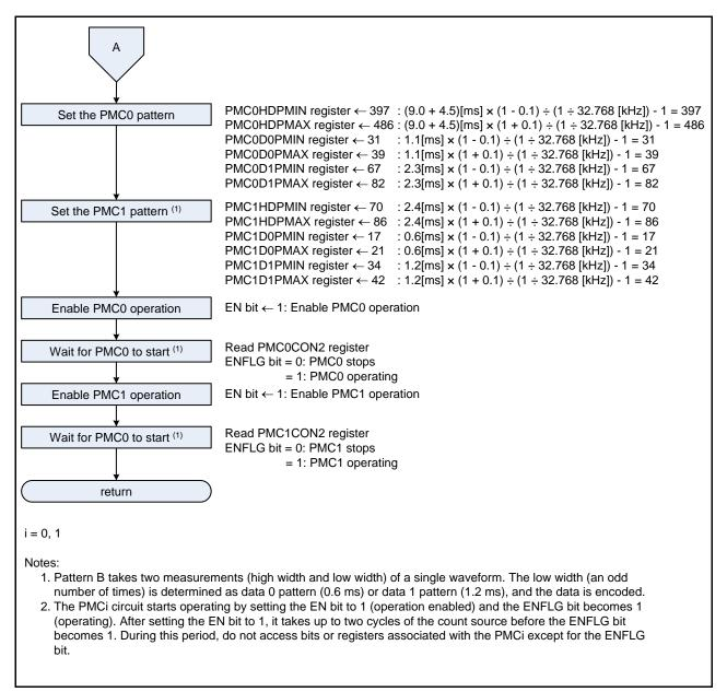
Figure 5.6 PMCi Initialization Processing (2/2)
