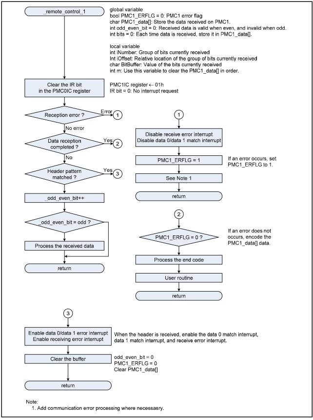
Figure 5.10 PMC1 Interrupt Handling
