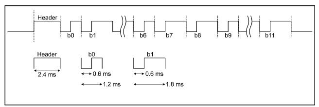
Figure 1.2 Pattern B: Remote Control Format with Special Header Pattern
