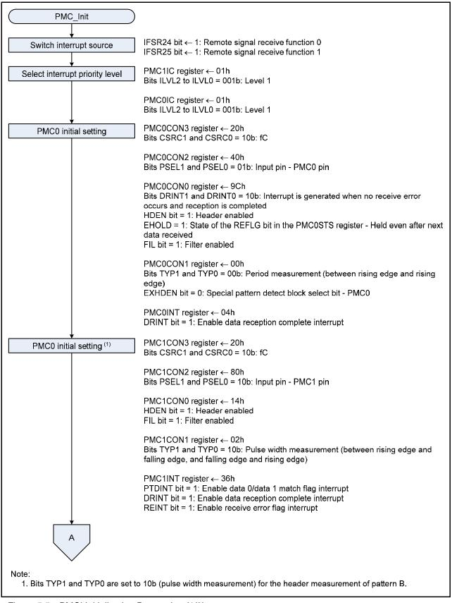
Figure 5.5 PMCi Initialization Processing (1/2)
