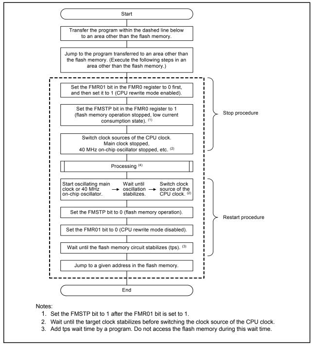
Figure 3.1 Stopping and Restarting the Flash Memory
