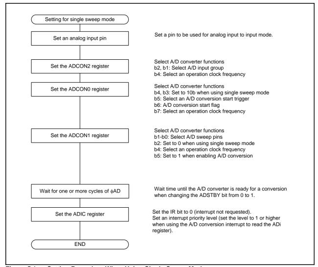
Figure 5.1 Setting Procedure When Using Single Sweep Mode
