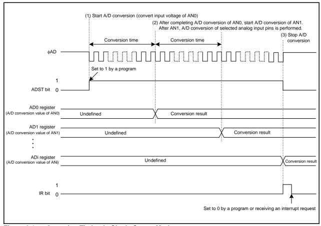
Figure 3.1 Operation Timing in Single Sweep Mode
