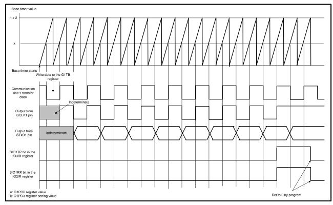
Figure 2. Transfer/Receive Timing Diagram of Communication Unit 1
