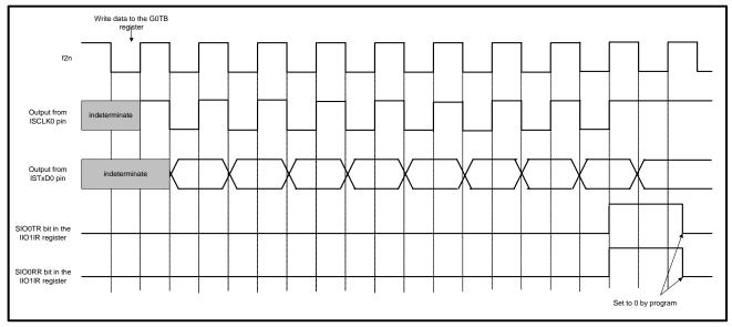
Figure 3. Transfer/Receive Timing Diagram of Communication Unit 0
