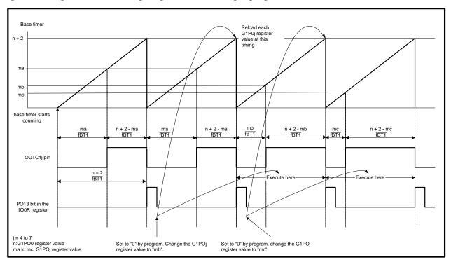
Figure 1. PWM Waveform Timing Diagram
