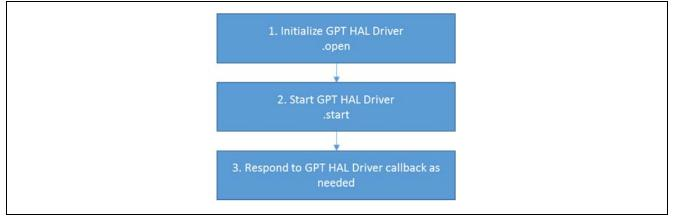
Figure 4 Typical GPT HAL Module Application Flow Chart
