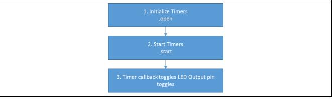
Figure 5 GPT HAL Module Application Project Flow Diagram
