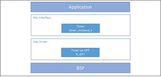
Figure 1 GPT HAL Module Block Diagram
