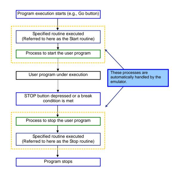
Actually, there exist some firmware processing before the user program actually starts running after execution of the Start routine is complete, and before the Stop routine is executed after the program has stopped in the above flow diagram.
