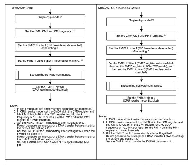
Figure 4.3 Comparison of Setting and Resetting of CPU Rewrite Mode (EW1 Mode)
