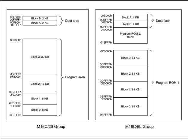
Figure 4.1 Differences in Flash Memory Block Structure
