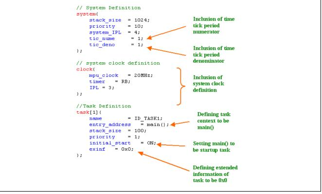
Figure 13 Enlistment of RTOS Resource in Template.cfg
