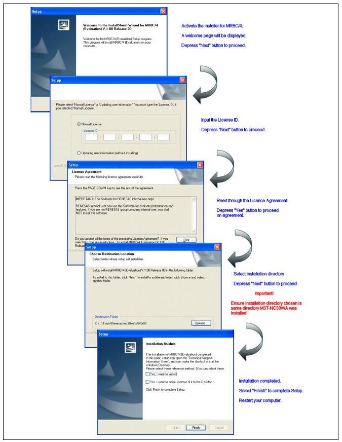
Figure 2 Procedures in MR8C/4 Installation
