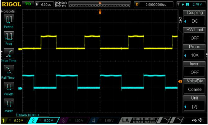
Figure 12 Period of the Schmitt Trigger Oscillator - 16.9 us
