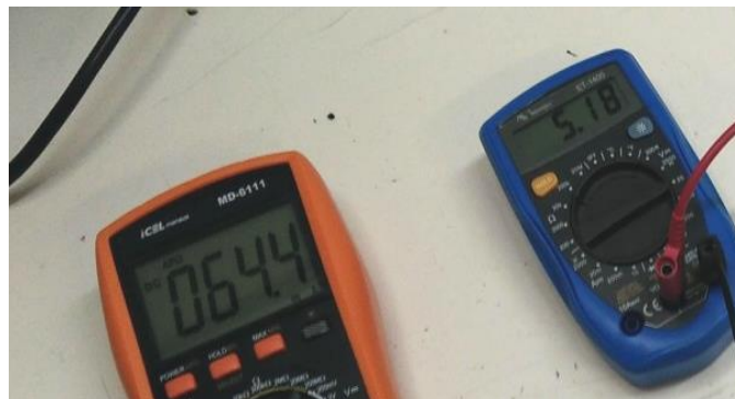
Figure 14: Measurement of Input Current and Output Voltage with Heavy Load
