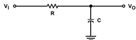
FIGURE 11. INTEGRATOR CIRCUIT
