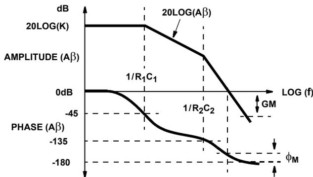
FIGURE 19. LOOP PHASE AND GAIN PLOT OF EQUATION 27
