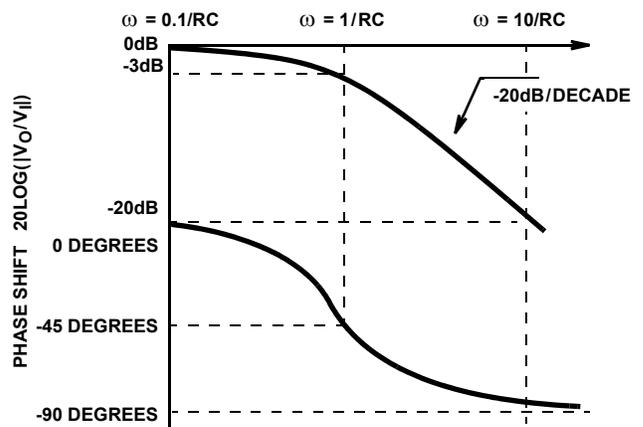
FIGURE 12. BODE PLOT OF INTEGRATING CIRCUIT TRANSFER FUNCTION
