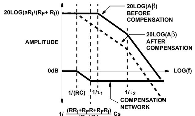
FIGURE 29. LEAD-LAG COMPENSATION SCHEMATIC AND  $A\beta$  AMPLITUDE PLOT
