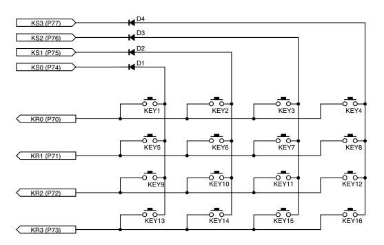
Figure 4-3. Key Matrix Circuit Diagram
