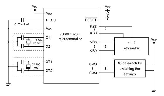
Figure 4-1. System Circuit Diagram
