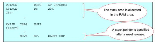
In this example, the address FFEE0H (= FFEC0H + 20H) is specified for the stack pointer. By using the above code, the last 32 bytes of the RAM area (FFEC0H to FFEDFH) can be allocated as the stack area.
