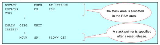
In this example, the address FFE20H (= FFE00H + 20H) is specified for the stack pointer. By using these settings, the stack area can be allocated while avoiding the saddr area.
