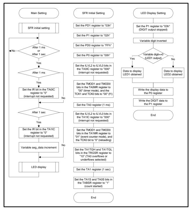
Figure 3. Register Setting Configuration
