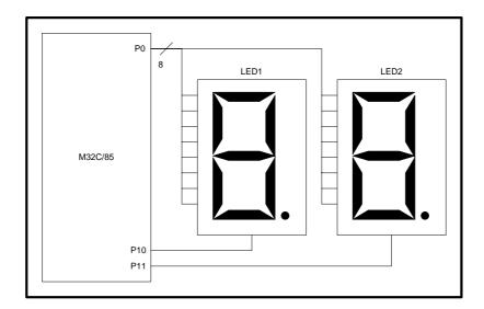
Figure 1. LED Block Diagram (1)
