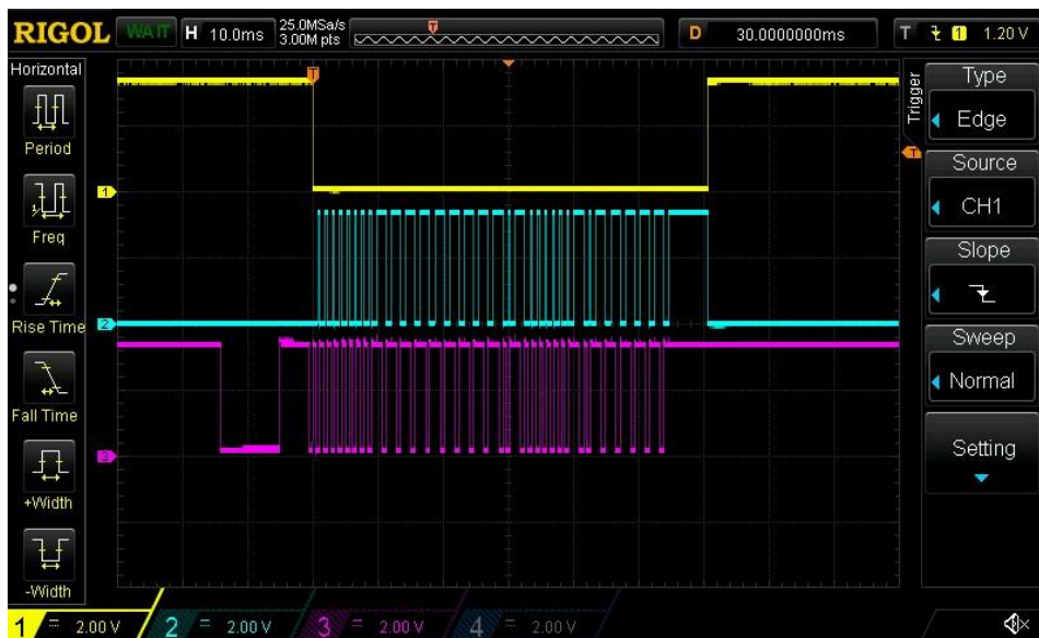
Figure 5. Conversion of the data stream from Serial to Parallel Channel 1 (yellow/top line) – PIN#14 (nCSB_OUT); Channel 2 (light blue/2 nd line) – PIN#5 (CLOCK_OUT); Channel 3 (magenta/bottom line) – PIN#12 (IR_IN)
