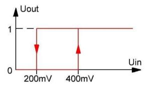
Figure 4. ACMP0 thresholds
