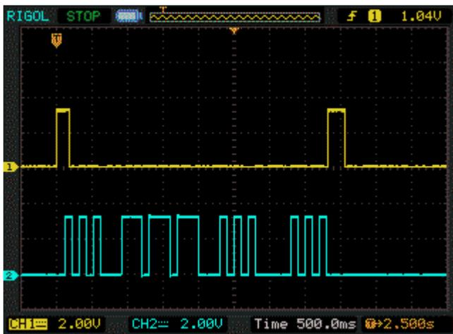
**Fig 3. SOS functionality waveforms**
