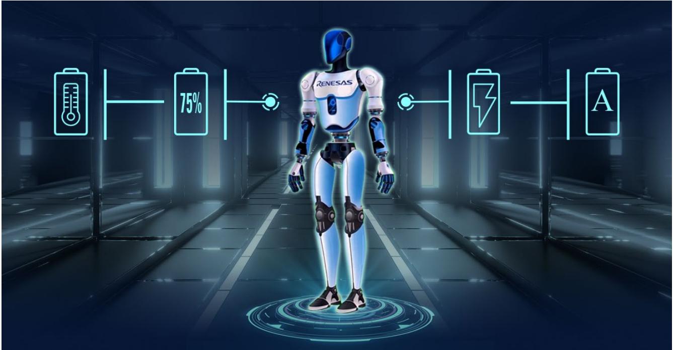
Figure 3: Humanoid BMS continuously monitoring battery voltage, current and controlling the battery pack temperature
