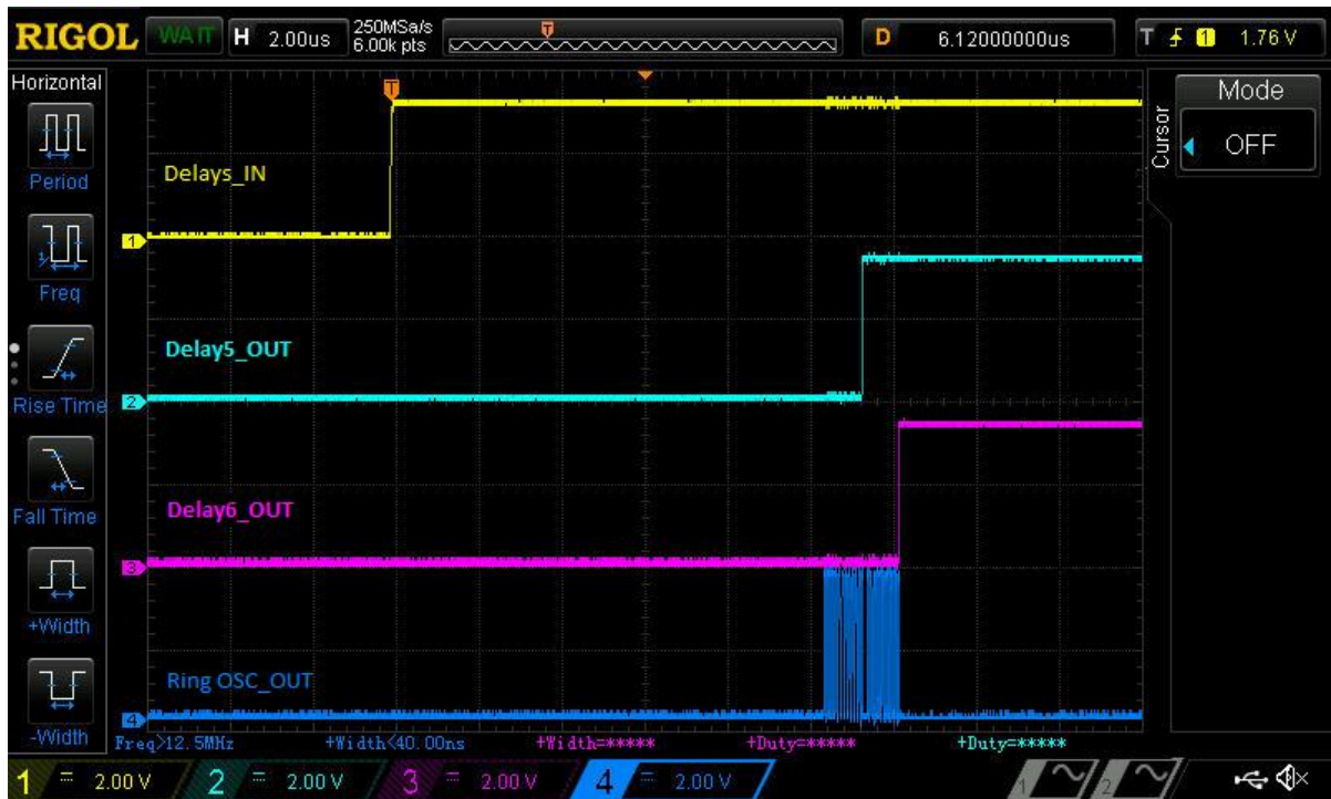
Figure 6. Ring OSC, DLY5 and DLY6 Waveform
