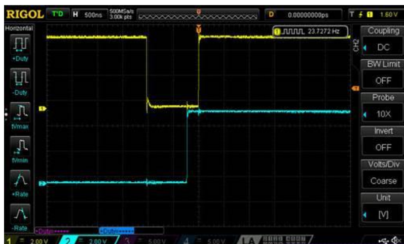
Figure 1. ACMP Output Glitch
