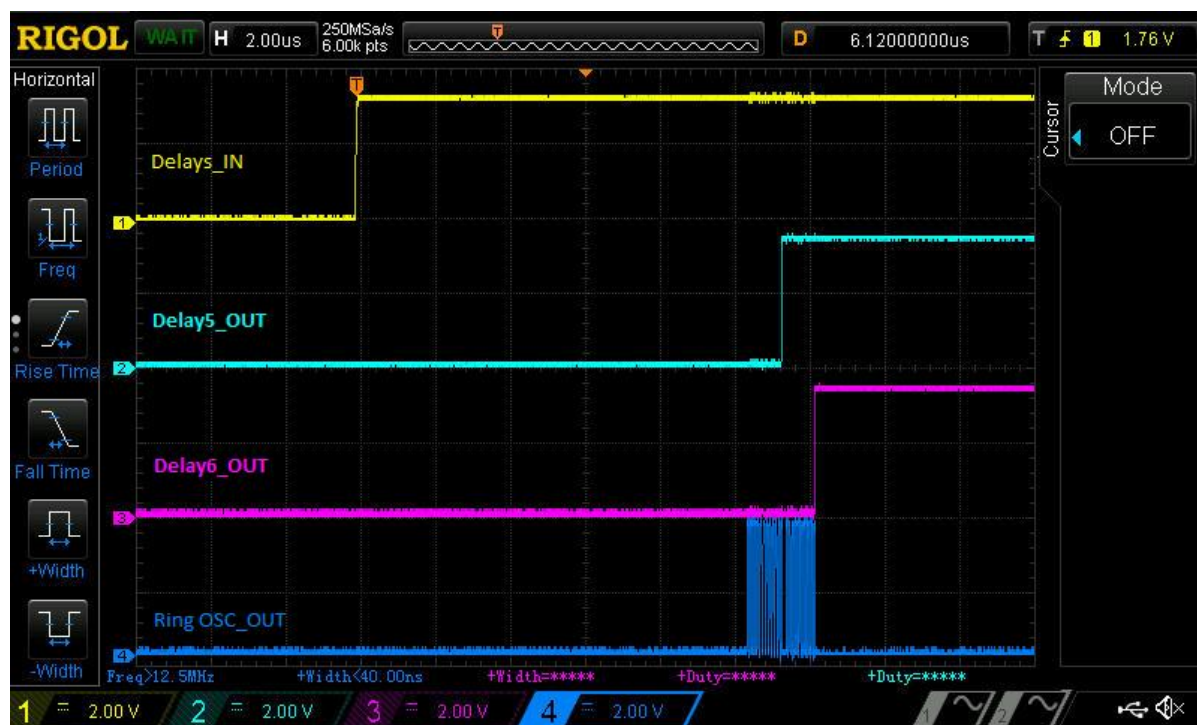
Figure 6. Ring OSC, DLY5 and DLY6 Waveform
