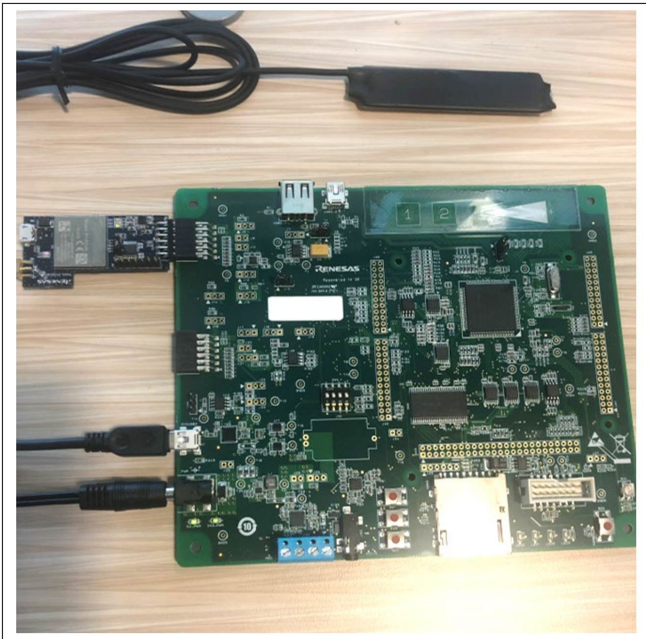
Figure 4. Connections for the RX671 Board After Flashing
