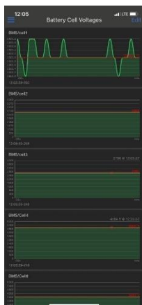
Figure 5-19. Graphical representation of Cell voltages vs time on IoT ON-OFF app
